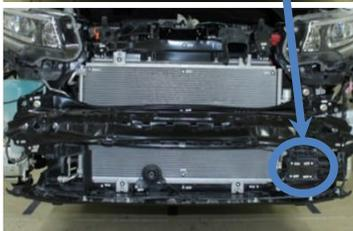
Example where damage to the radar sensor did not occur during the D&R test at Jiken center.
