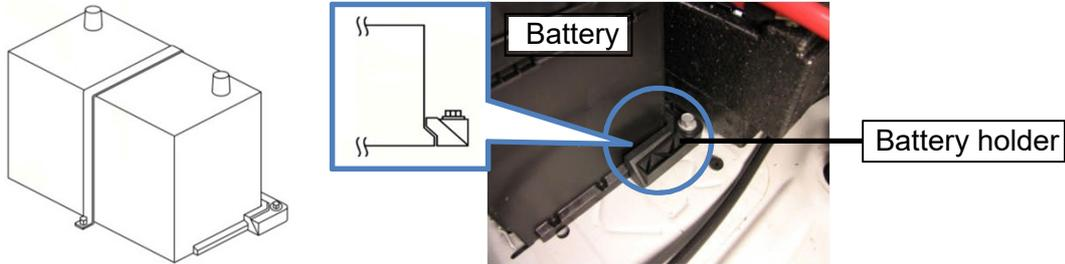
Example where the battery is secured in a way that it does not move on impact.
