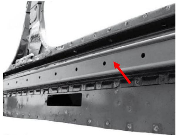
Sill reinforcement is a single piece and when damaged will require sill cover removal and sectioning.
