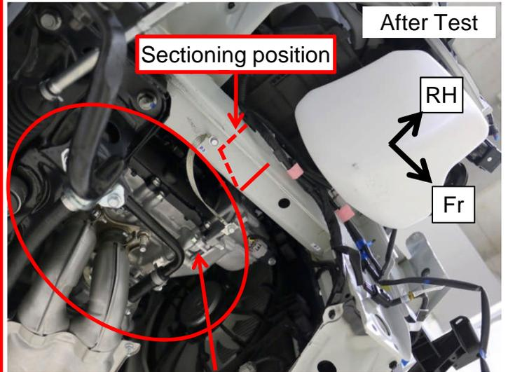
Engine must be removed for sectioning.
