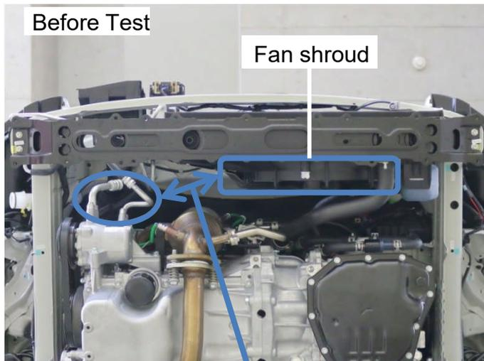
The fan shroud is offset and clearance between the fan shroud and the air conditioner condenser pipe is large.
