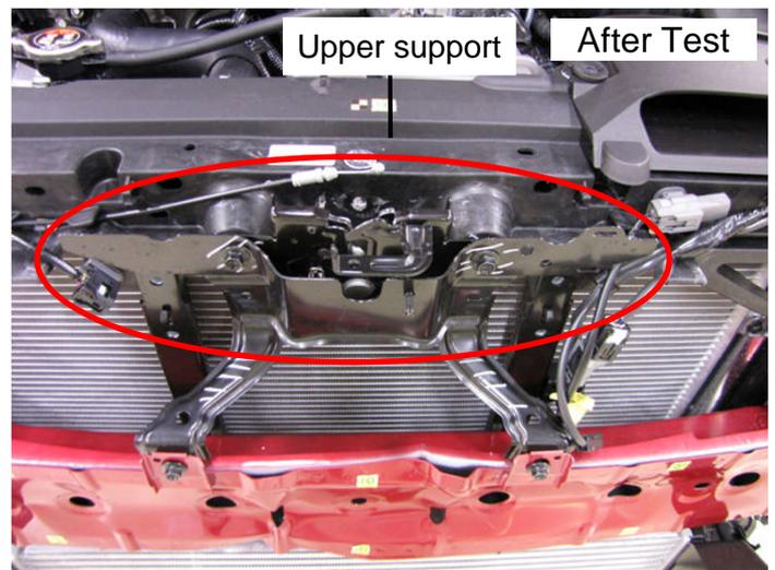
Hood lock is installed in front of the upper support.
