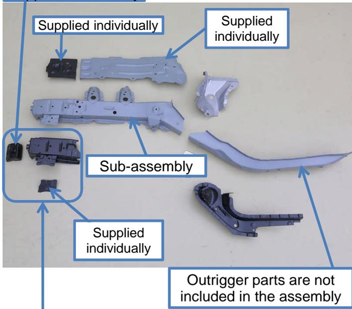
The front side is not included in the assembly, which eliminates the need for sectioning and splice welding.
