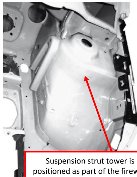
Suspension strut tower is positioned as part of the firewall plenum chamber and the front inner wing.
