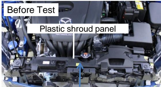
Shroud panel is detached from the mount on the body to protect the unit in a collision.
