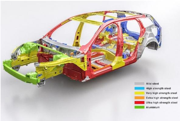
The parts made of Ultra High Strength Steel are clearly indicated.
