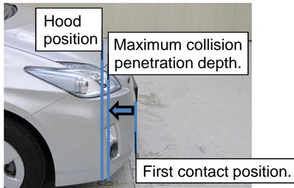
Example where the distance from the front end of the bumper to the front end of the hood is longer than the maximum collision penetration depth.
