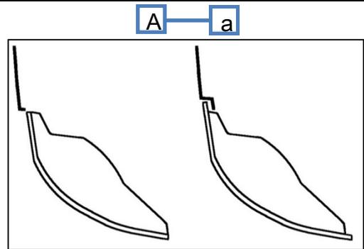
Example of a shape where the headlight is less likely to interfere with the fender.
