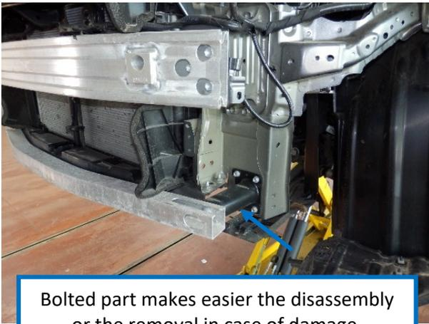
Bolted part makes easier the disassembly or the removal in case of damage.
