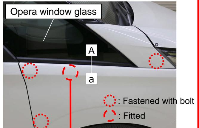
The front fender is not directly fixed to the opera window glass, which allows the fender to expand to the outside, causing the molding lip to get caught in the fender.
