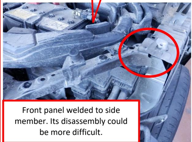
Front panel welded to side member. Its disassembly could be more difficult.
