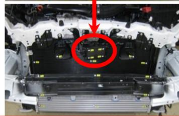
Installed on the back side of the bumper cover. Damage to the radar sensor occurs when pressed.
