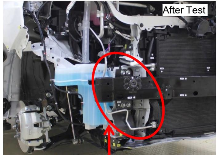
Front section of the pipe was damaged.
