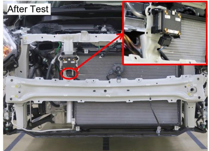
The auto brake controller connector was damaged.
