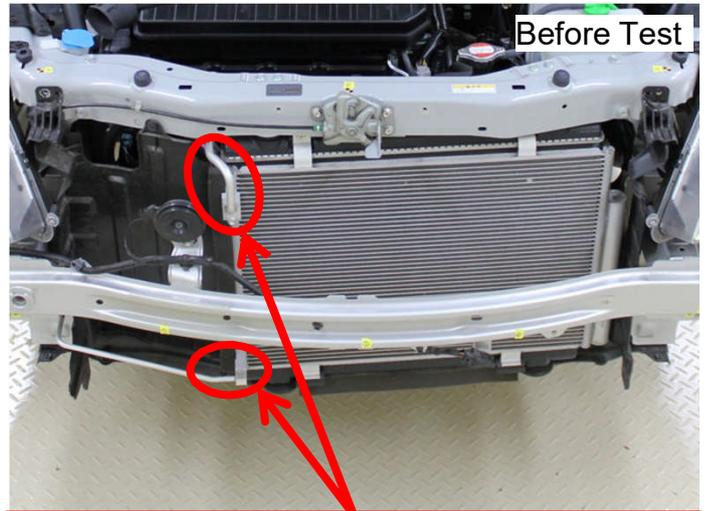
Two air conditioner condenser pipes are installed very close to the bumper
