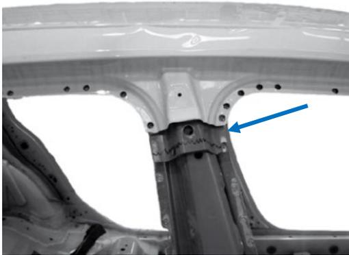
B' Post can be sectioned through reinforcements and both index outer and closing panel without having to cut into upper roof rail. Most reinforcements made from UHSS cannot be sectioned.
