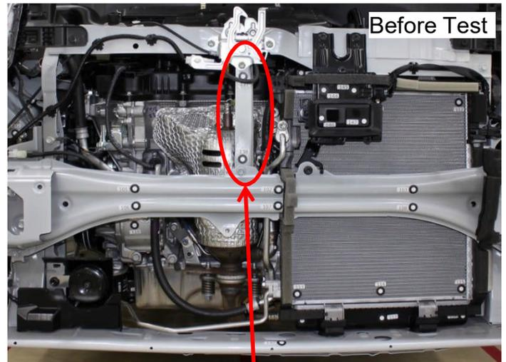
The hood lock support at the front of the exhaust manifold converter is weak.
