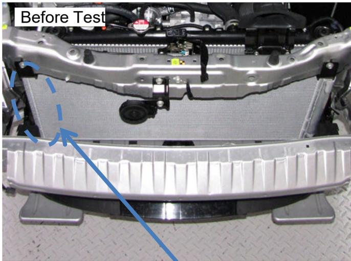
The air conditioner condenser pipe is installed behind the condenser.
