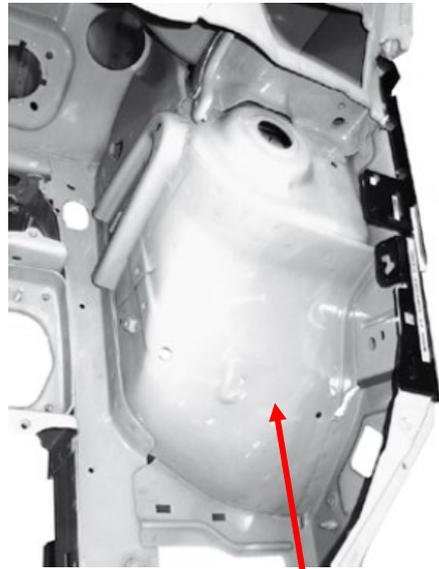
Strut tower is a unique part. Repair requires completely replacement.
