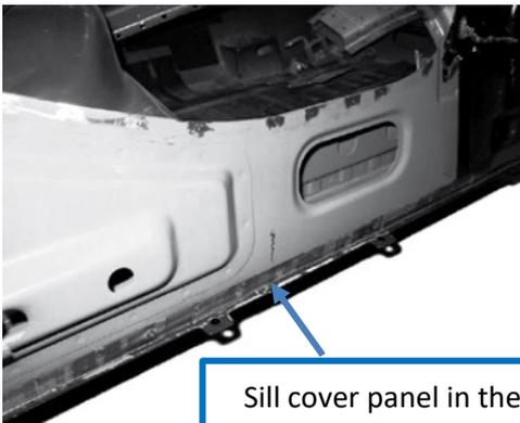
Sill cover panel in the rear reinforcement.
