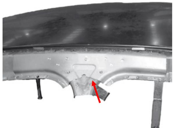
'B' Post has to be sectioned and roof rail has to be opened for the reinforcement to be fed between panels.
