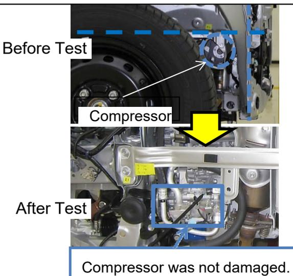
The compressor is located behind the front end of the side member but overlapped inside of the horizontal surface of the side member.
