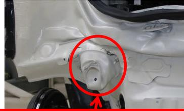
Crush box fell over at an angle.
