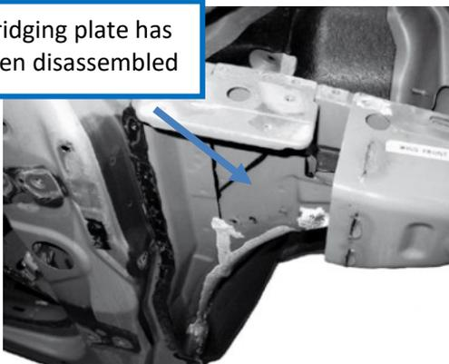
Bridging plate creates a joint between 'A' Post and side panel reinforcement, easing removal of both panels.
