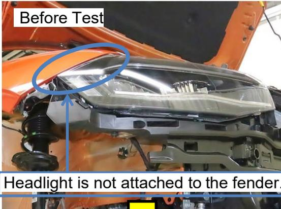
Headlight is not attached to the fender.
