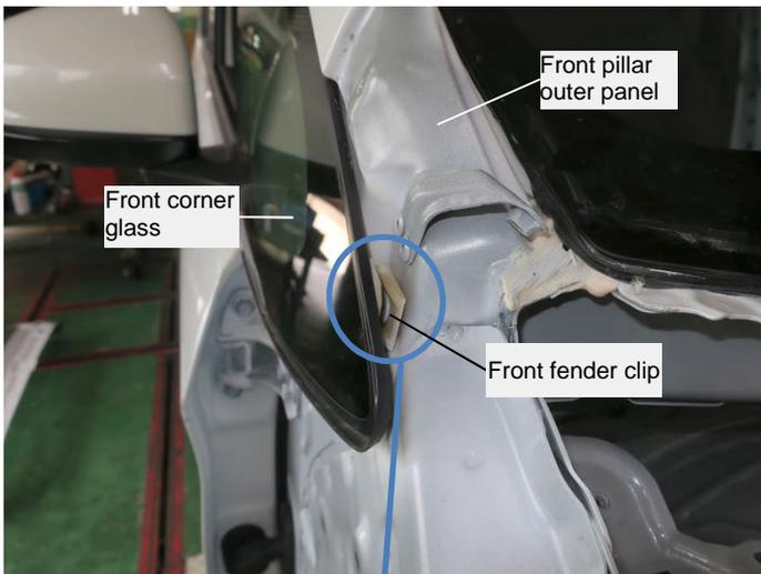
The front fender is securely fixed to the opera window glass with the fender clip, which helps prevent the fender from expanding to the outside in a collision.
