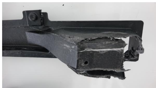
The bumper reinforcement was broken
