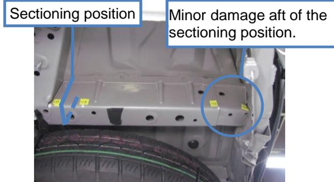
Example of a structure that allows damage to end aft of the sectioning position of the rear side member.
