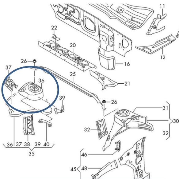
The strut tower is a separated part from the front inner wing.
