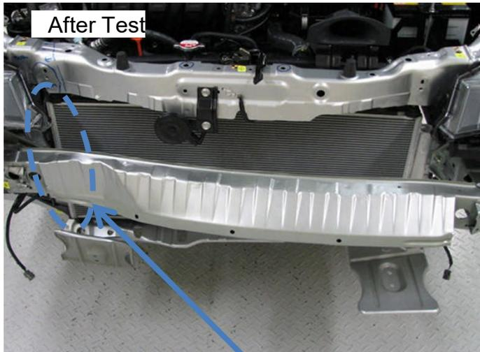
Air conditioner condenser pipe was not damaged.
