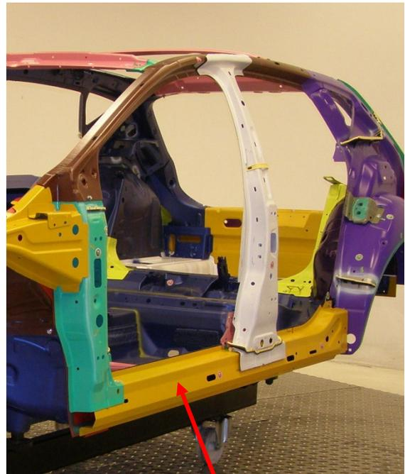
Sill reinforcement is a single part and when damaged will require sill cover removal and sectioning.
