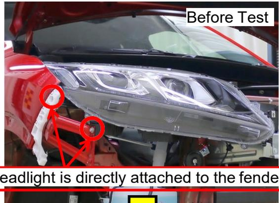
Headlight is directly attached to the fender.
