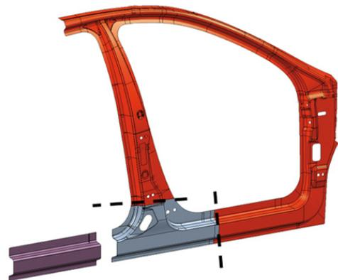
'A' Post reinforcement is a unique part. Its removal required its complete disassembly.
