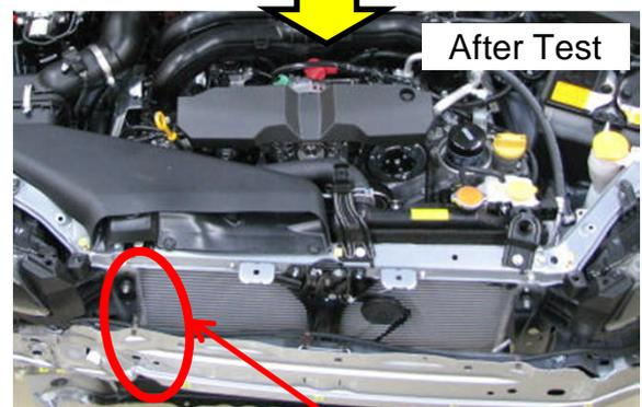
Condenser was bent and damaged.
