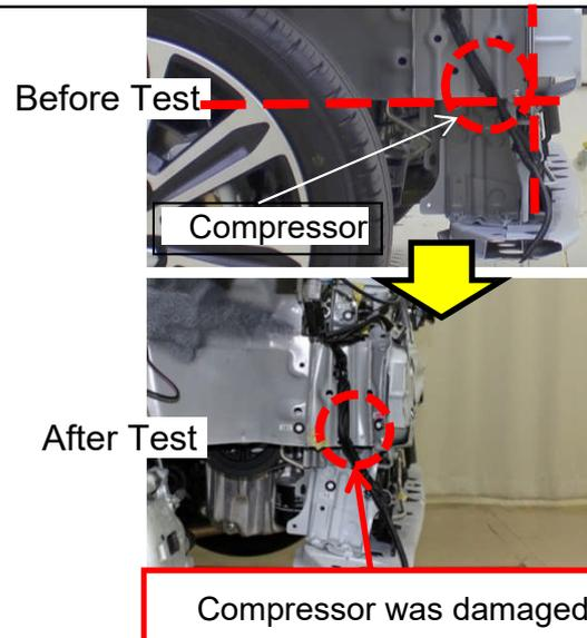
The compressor is located behind the frontend of the side member and outside of the horizontal surface of the side member.
