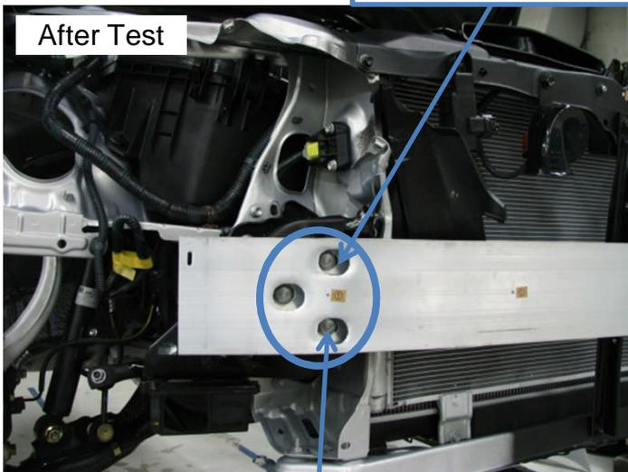
Easy to remove because the bolts do not bend easily.
