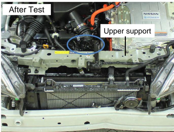
Hood lock is installed behind the upper support.
