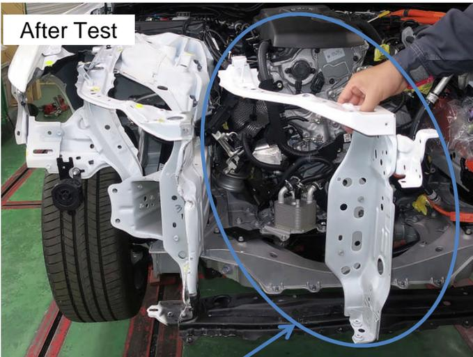
Only the damaged right side support was replaced.
