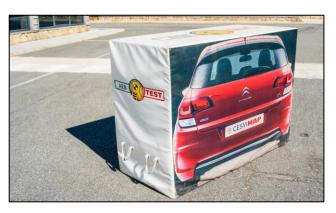
Figure 2 – CESVIMAP vehicle target
