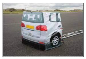
Figure 3 – Euro NCAP Vehicle Target (EVT)
