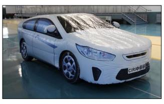
Figure 4 – CIRI inflatable vehicle target
