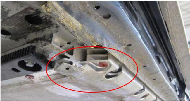
Figure 1: Damaged battery housing
