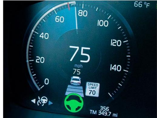
ACC and partial automation systems on the market today don't restrict drivers from setting speeds that are higher than the legal limit. When selecting a speed to "set and forget," many drivers choose one over the limit.
