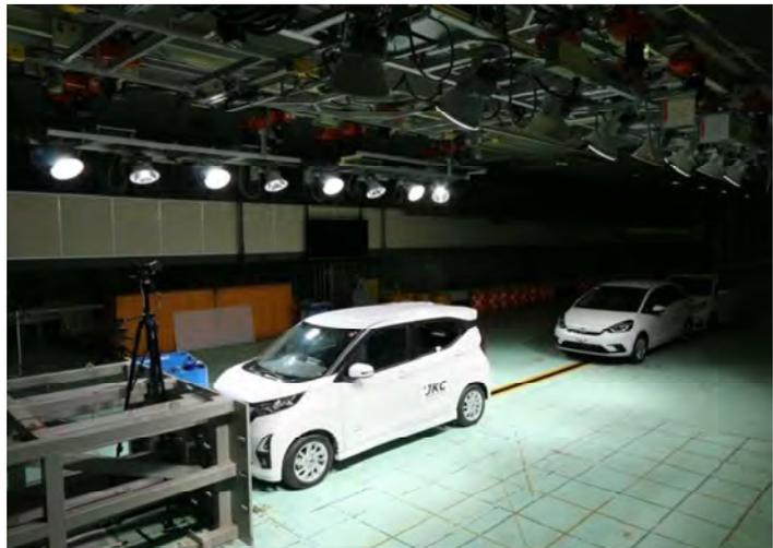
With the new lighting system, lightings can be divided into two parts, front and rear. Therefore, in the multiple crash test, sufficient illumination can be provided to the second (crashing) vehicle.
