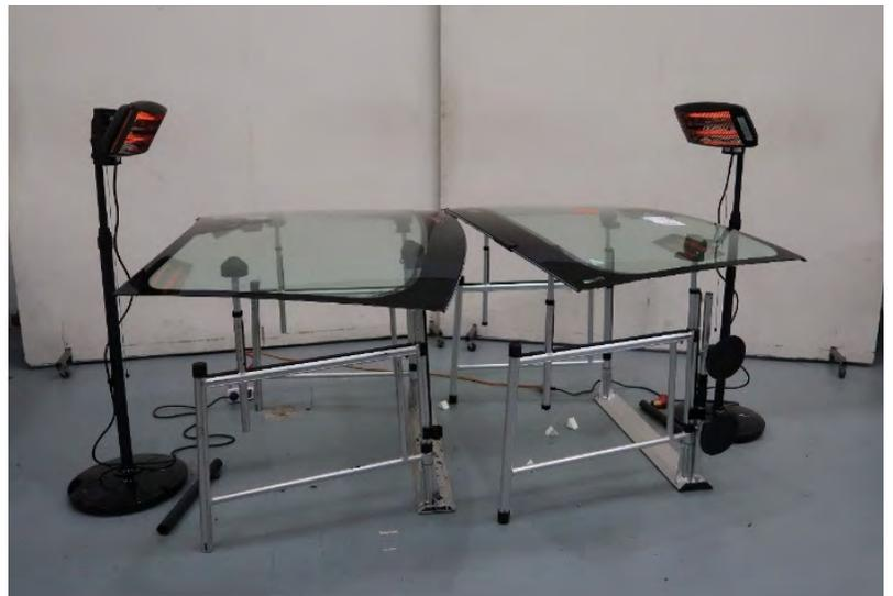
Image: Windscreen controlled heating arrangement
