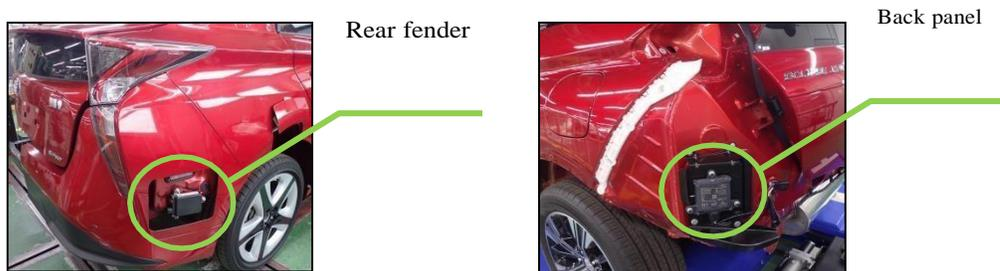
Displaced position of the sensor is likely to affect its effectiveness of radio wave irradiations (See the images below).
