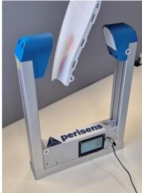
Device for measuring one-way damping (dB), Source: Perisens
