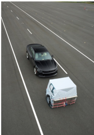
The original IIHS vehicle-to-vehicle front crash prevention test
