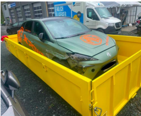
Overcautious quarantine storage of BEV after collision with guiding rail
