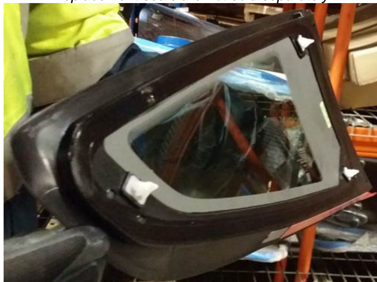
There are also locating pins which are sheared off when removing side glass.
