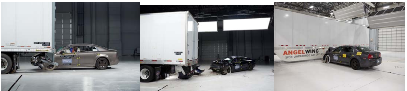
Photos: Great Dane semitrailer rear underride guard test AngelWing side guard test
