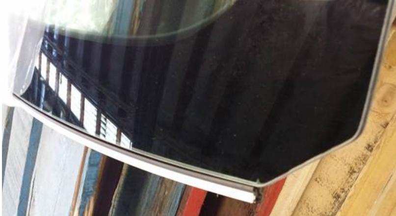
The windscreen has bonded seals which are damaged when the windscreen is removed
