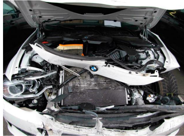
Fig. 2: Expensive cosmetic parts destroyed but crash management system mainly unaffected
