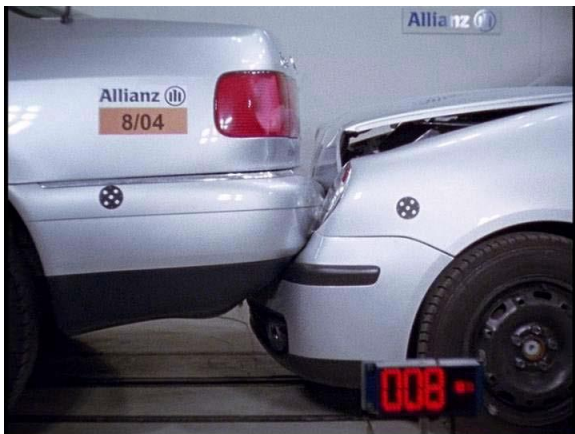
Fig. 5: No bumper interaction in car-to-car crash, underride
