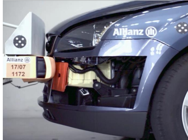
Fig. 10: Limited intrusion with appropriate bumper performance, net repair costs 1,130 EUR
