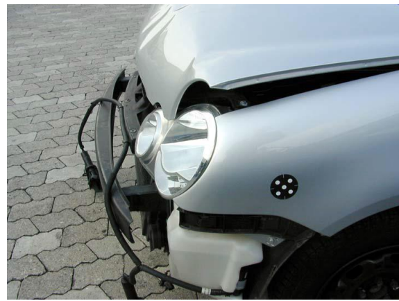
Fig. 6: Crash management system not affected, unnecessary damage
