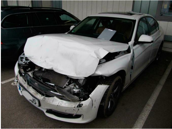
Fig. 1: Typical damage after underride
