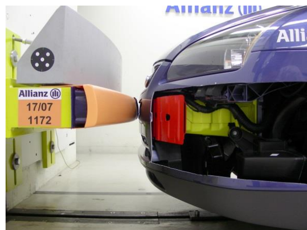
Fig. 8: Appropriate bumper alignment, cut-out in bumper fascia for visualization
