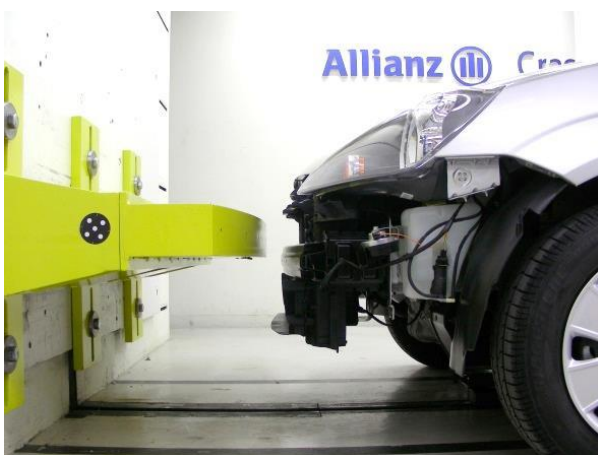
Fig. 7: RCAR Bumper Test with poor bumper alignment
