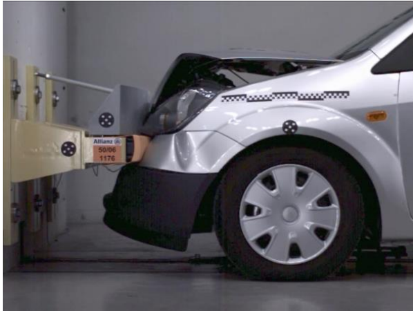
Fig. 9: Deformation with poor bumper alignment, here: underride, net repair costs 2,760 EUR
