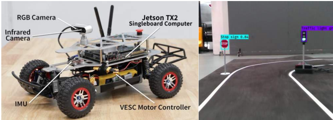
1/10 Scale Autonomous Vehicle and Screenshot of Object Recognition and Classification Engine
