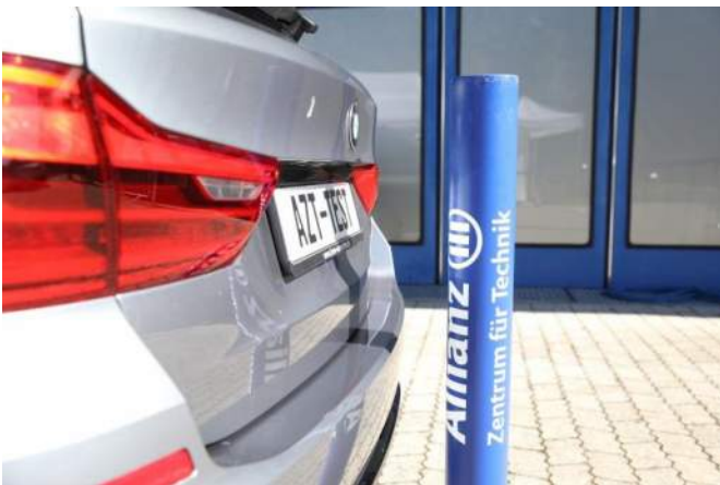
Reverse AEB - test with bollard as test object
