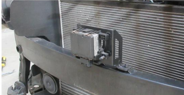
Radar Sensor on a thin bracket in a vulnerable position
