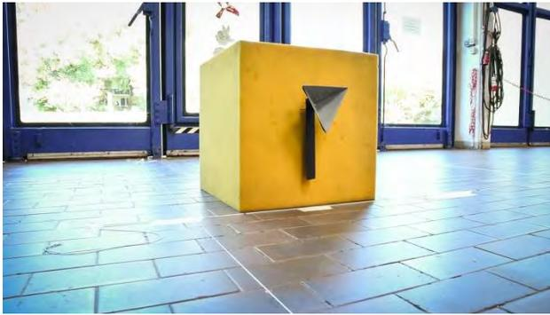
*Example of a tool for front radar calibration*
