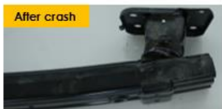
Tow hook located side the crush cans of the rear beam
