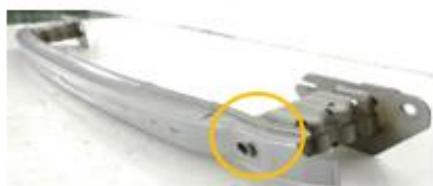
Tow hook located into crush cans of the rear beam.
