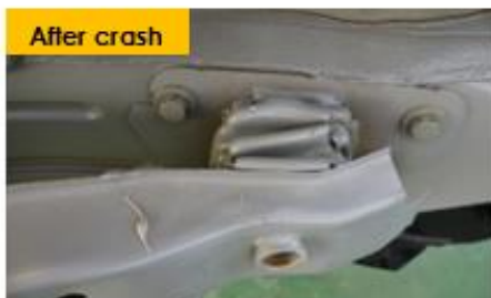
Tow hook located into crush cans of the rear beam.
