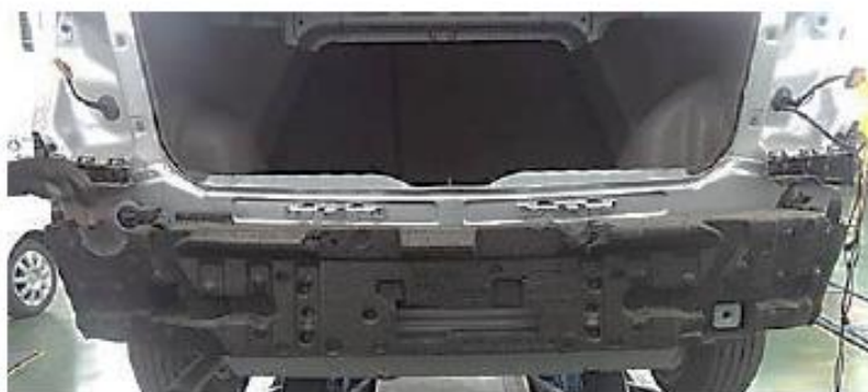
Only polystyrene mounted on the rear panel
