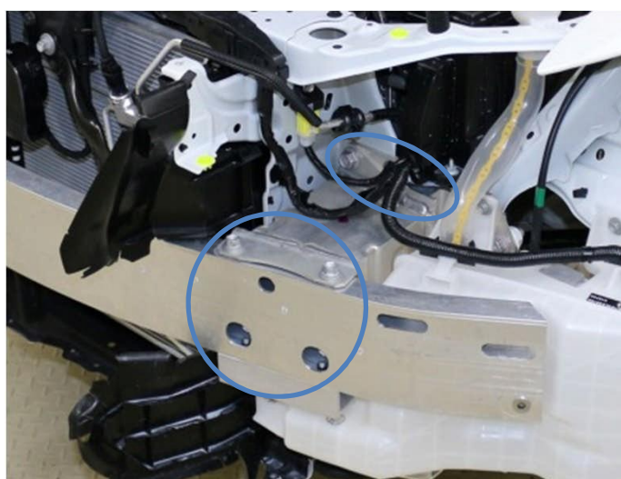
Example where stud bolts are not used
