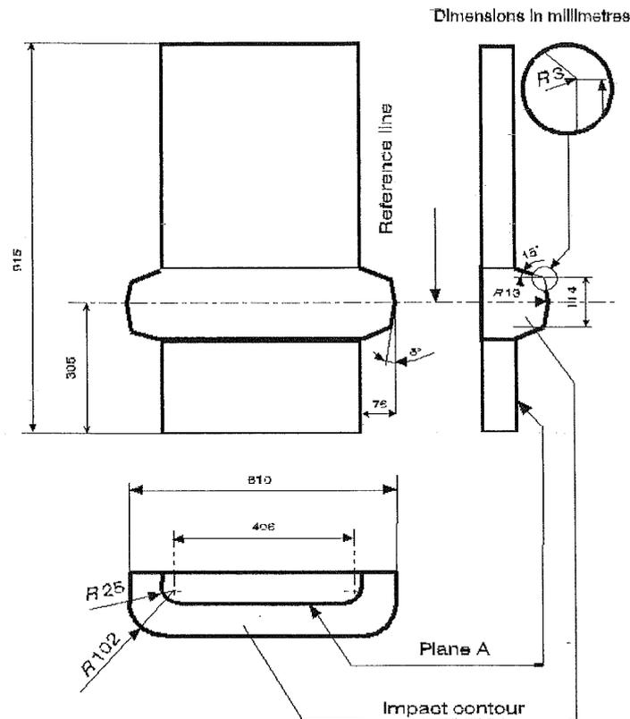
The impactor axis height is to be 445 mm from the ground surface, both for front devices and rear devices.
