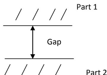
B) Parallelisms. The outlines of two adjacent parts usually should be parallel to each other, that is to say, a continuous distance from each other.
