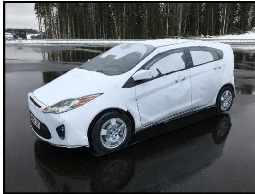
Figure 1 – Global Vehicle Target (GVT)
