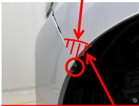
The ends are fastened with screws, so the fender would also be damaged.
