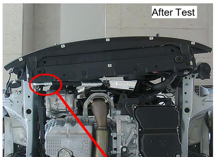
The fan shroud and air conditioner condenser pipe were damaged.
