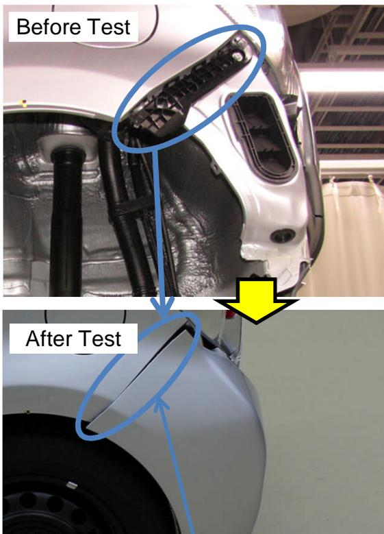
The fender and bumper cover were just fitted together and could be easily detached, which prevented damage to the rear fender.
