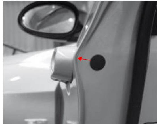
A door-skin with the curvature inwards makes it difficult to repair and paint.
