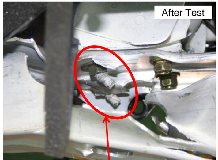
Nuts cannot be removed due to bent stud bolts.
