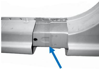
'A' Post cover and reinforcement where it joins the sill which are sectionable, making removal of the 'A' Post reinforcement easier and allowing for sectioning of the sill.
