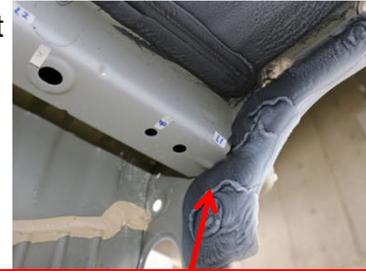
Rear end of the side member does not have reinforcement and is weak.
