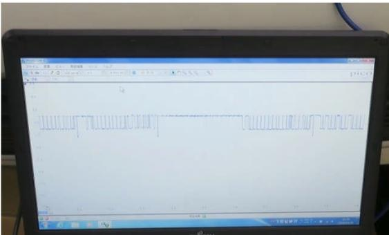
Whether or not the millimeter-wave radar is radiating correctly can be checked with the oscilloscope function of a PC with a diagnostic device installed.
