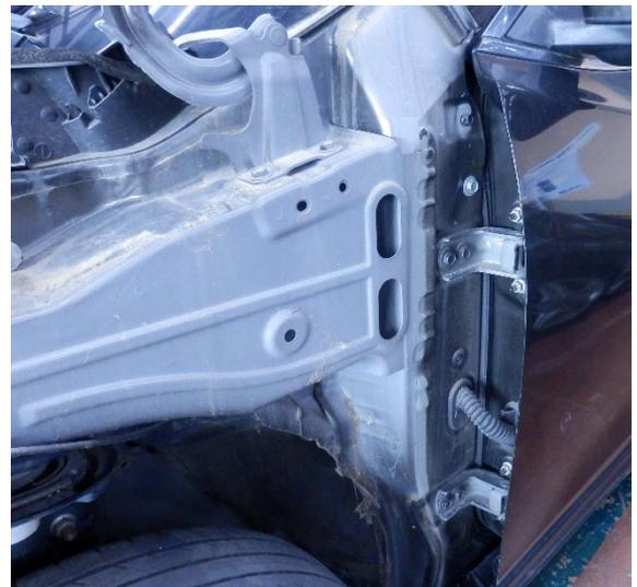
'A' Post reinforcement is a unique part. Its removal required its complete disassembly.
