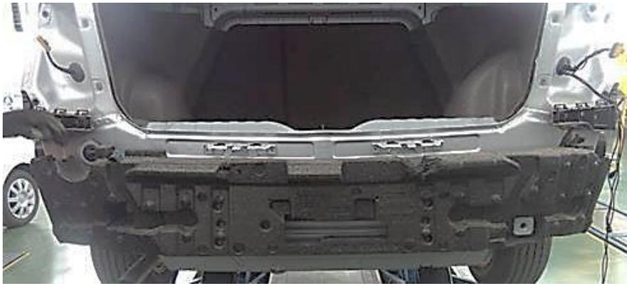
Only polystyrene mounted on the rear panel
