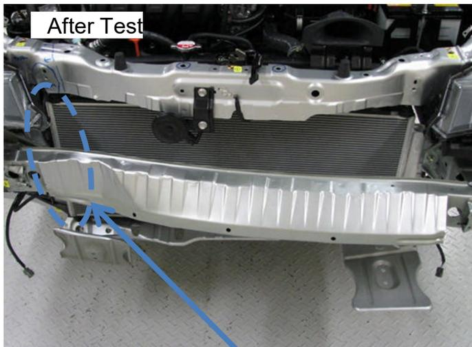
Air conditioner condenser pipe was not damaged.
