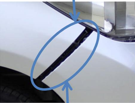
The fender and bumper cover are just fitted together and can be easily detached, which prevented damage to the rear fender.
