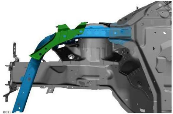
Intrusive requirement to remove A Pillar outer section
