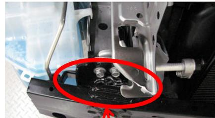
Crush stroke is too short for the crush box to absorb all of the crash energy.
