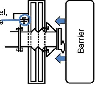
Example of a structure where the condenser and radiator slide rearward together with the shroud panel that moves rearward when the crush box crushes in a collision.
