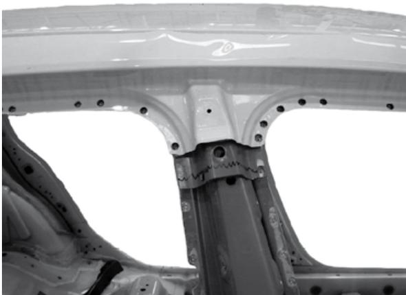
'B' Post can be sectioned through reinforcements and both outer and closing panel without having to cut into upper roof rail. Most reinforcements made from UHSS cannot be sectioned.
