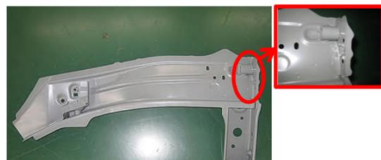
The front end part is supplied with side member as an assembly, so it had to be removed from the assembly.
