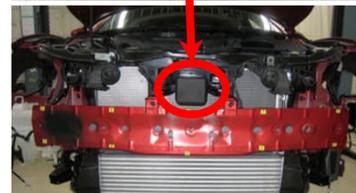
Installed on the back side of the bumper cover. Damage to the radar sensor occurs when pressed.
