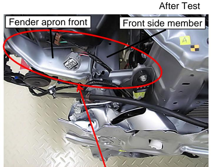
Damage to the fender apron front occurred when the side member was damaged.
