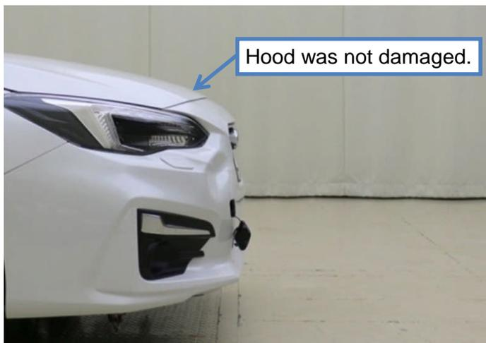
The hood was not damaged because the front end of the hood was higher than the barrier back stop.
