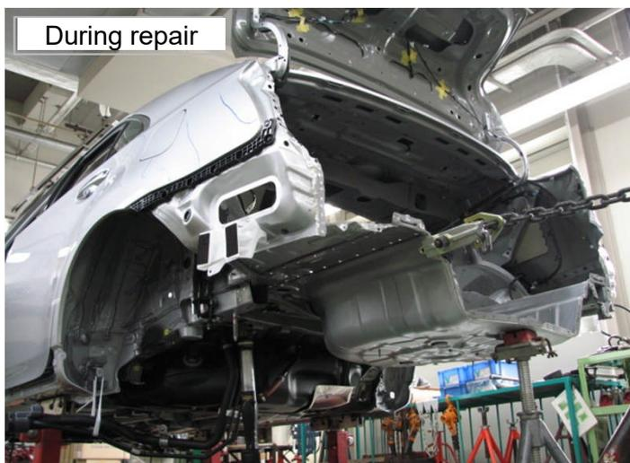
Removal of the fuel tank was not necessary as the fuel neck is separate from the fuel tank.
