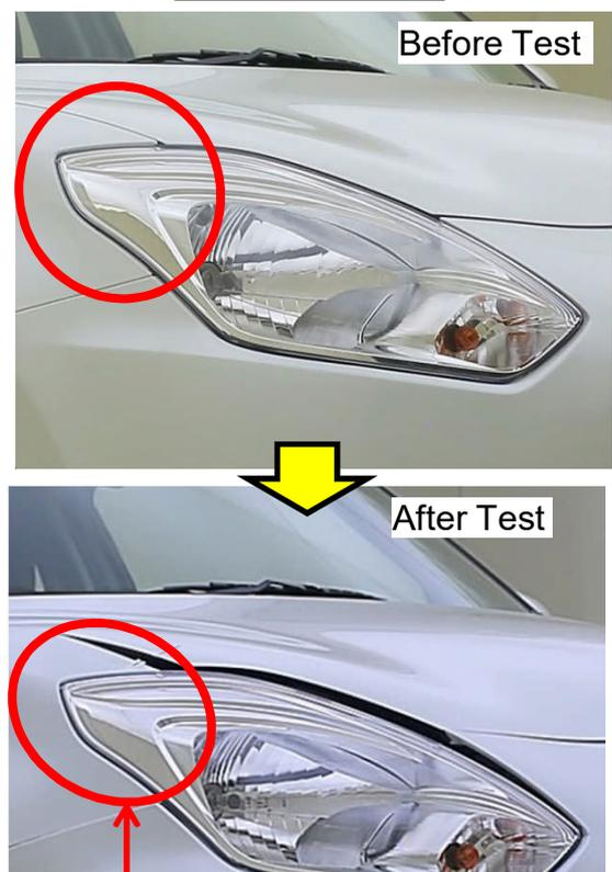
Due to the structure that allows the headlight to interfere with the fender, damage to the fender is likely to occur in a collision.
