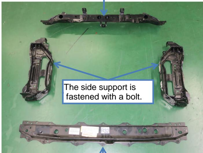
The side support is fastened with a bolt.
