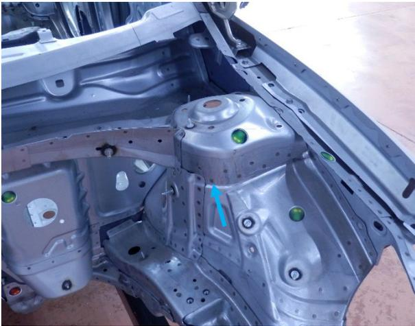
Strut tower has been fitted to the body using spot weld. Any evidence of repair could be removed.
