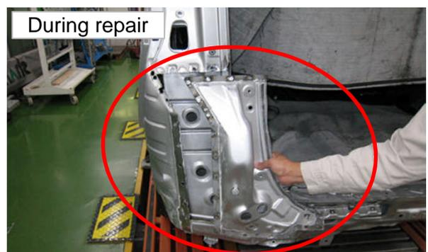
The adjacent panels had to be removed because the rear panel was installed in the inner position.
