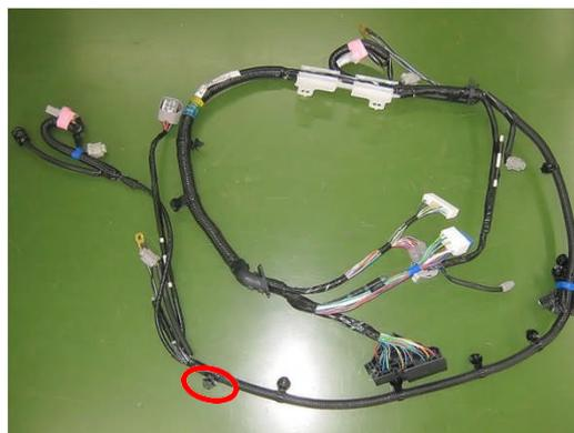
Only the harness clip was damaged, but the harness assembly had to be replaced as the harness clip is not supplied individually.
