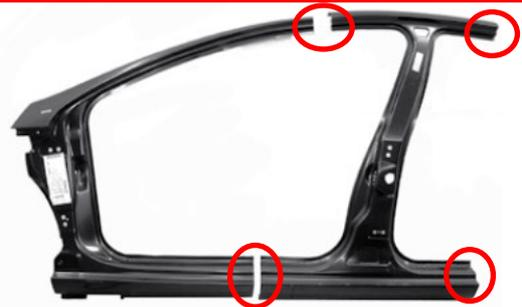
Service parts supplied in separate units need joining up when fitting, unless the part covers the damage area.
