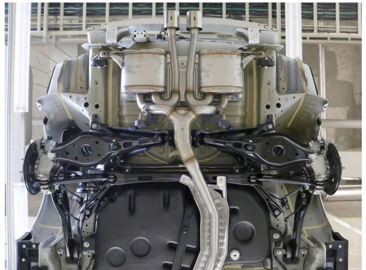
Middle pipe, rear muffler, and muffler finisher are supplied as an assembly.
