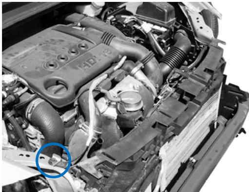
On impact the panel has broken, allowing parts fitted to the panel to move but not to be damaged.
