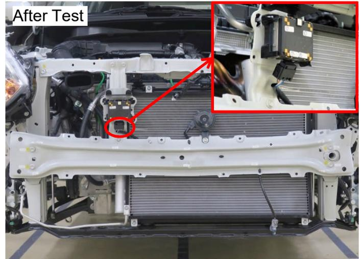
The auto brake controller connector was damaged.
