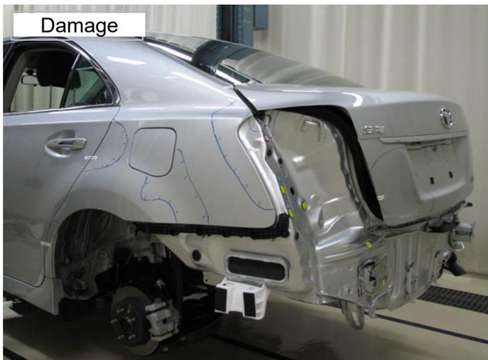
The quarter panel and rear side member were damaged and needed to be repaired.
