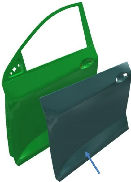
The door-skin is supplied as a separate part. In case of damage, only door-skin is removed
