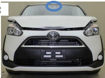
Installed on the windshield where damage to the radar sensor is less likely to occur. (Example where LIDAR is installed)
