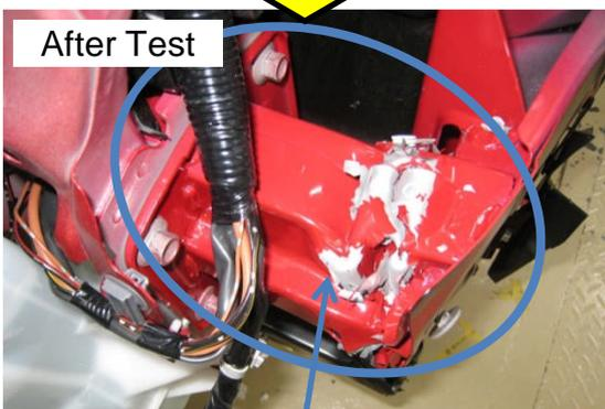
Crash energy was absorbed by the crush box. (Side member was not damaged.)
