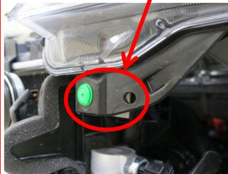
The bumper cover and grille are attached to the headlight. Damage to the headlight is likely to occur.
