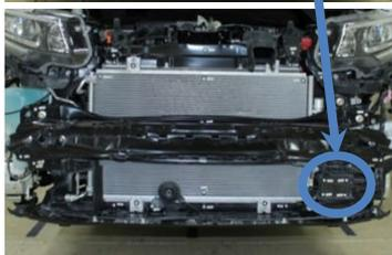
Example where damage to the radar sensor did not occur during the D&R test at Jiken center.
