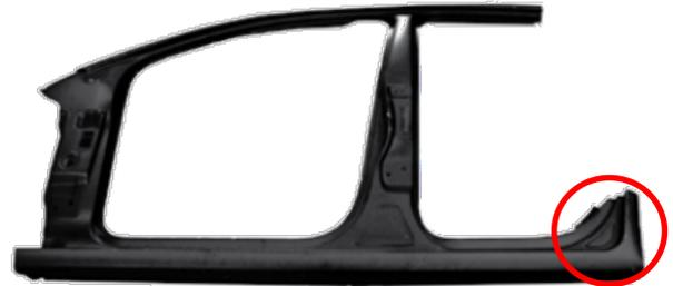
Service parts supplied as a side panel segment but having a joint at one of the most vulnerable and most frequently damaged parts like the dogleg.
