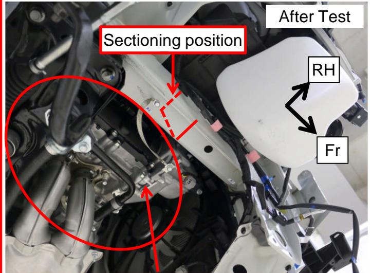
Engine must be removed for sectioning.
