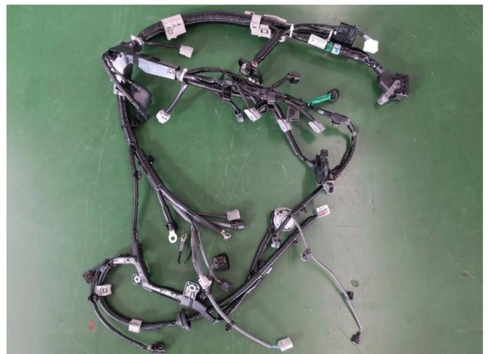
The main harness assembly had to be replaced as the auto brake controller connector was not supplied individually.
