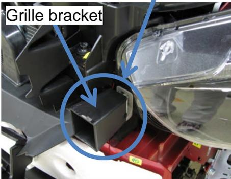
The grille bracket would be sheared off, which helps prevent damage to the headlight.
