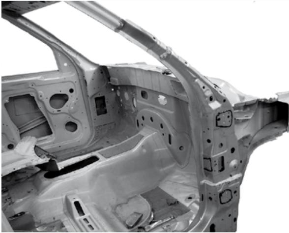
'A' Post reinforcement is sectionable at natural joint in upper part, avoiding complete removal.
