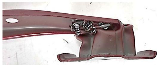
**Note:** The design and the material of the bumper reinforcement produces a good deformation that absorbs the energy of the crash.
