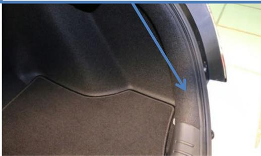
The quarter trim was not damaged because it does not extend to the tailgate opening.
