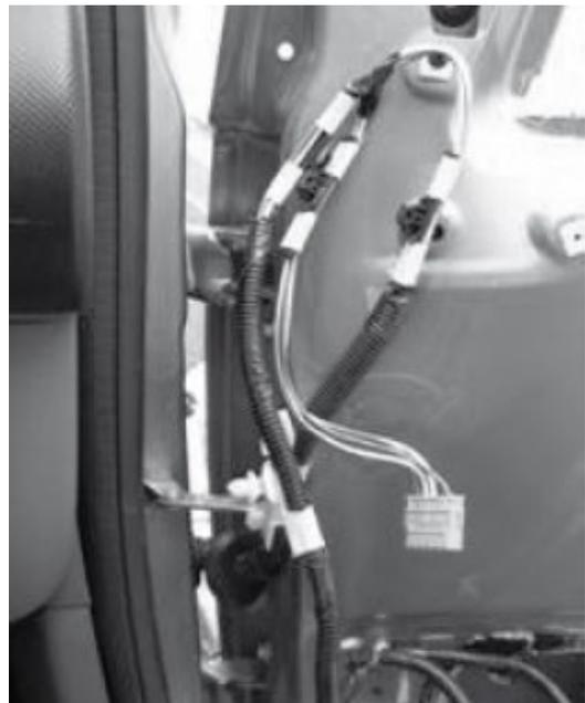
The door does not have a central electrical multi-connector, so it is necessary to remove the door trim and to disconnect the different electrical devices.
