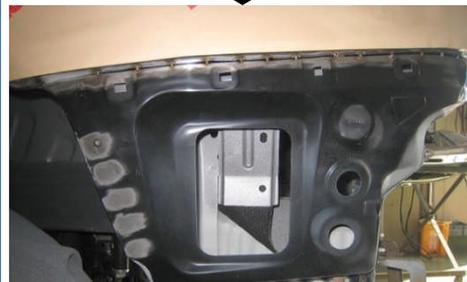
Only the lower section of the rear quarter panel was cut off and replaced (sectioning).
