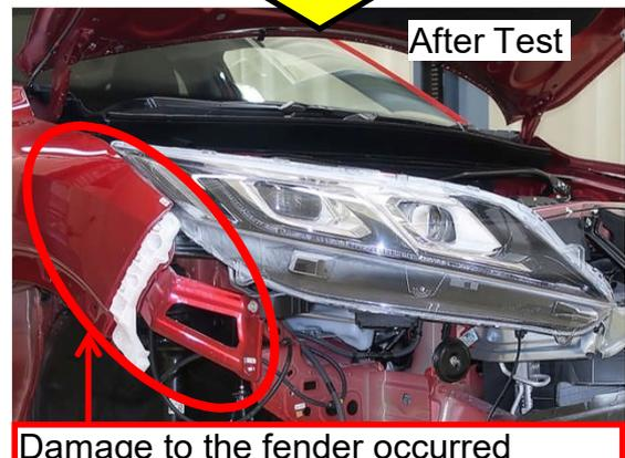
Damage to the fender occurred mainly around the attached area.
