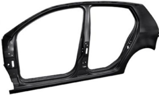
Service parts supplied as a whole that can be cut where required to suit the damage to the vehicle. This avoids any mismatching joints.
