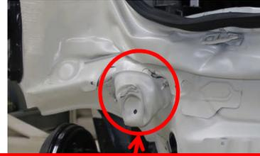
Crush box fell over at an angle.
