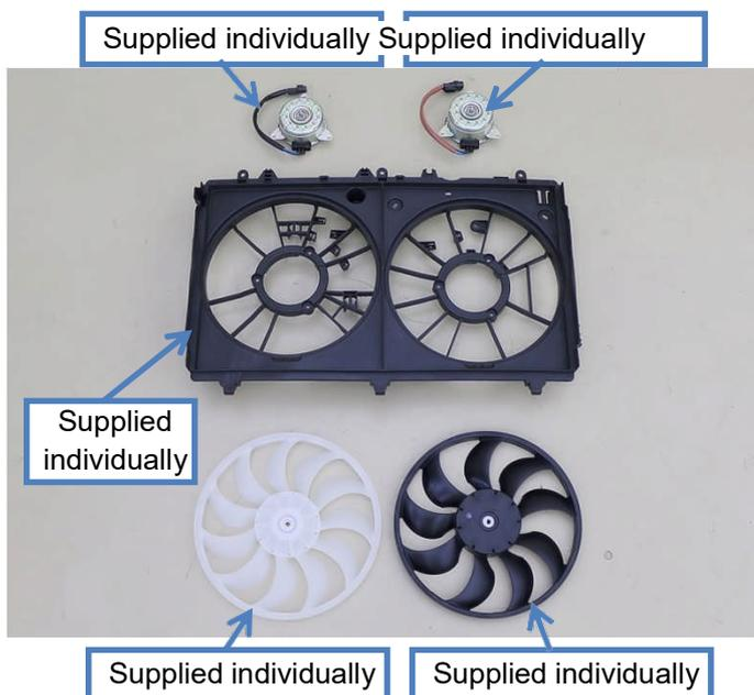
Parts are not supplied as an assembly but all parts are supplied individually.
