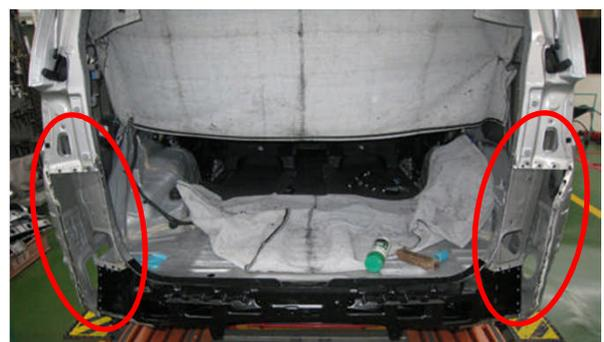
The left and right adjacent panels were removed so that the rear panel could be replaced.
