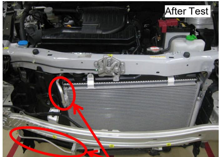
Air conditioner condenser pipe was pushed and damaged by the bumper cover.
