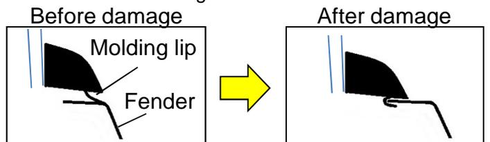
Molding lip goes inside of the front fender when the fender expands.
