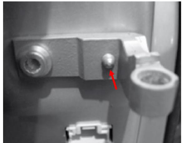
The access to the bolt causes problems in the repair. It is necessary to access from inside bodyshell, increasing the labour time.
