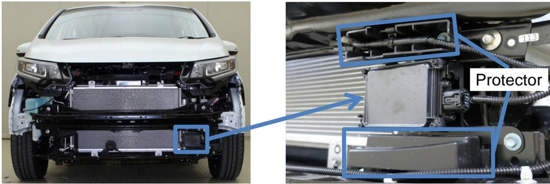
Example where the radar sensor is protected with a protective
