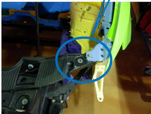
Front panel is a bolt-on part. Its disassembly is easier.
