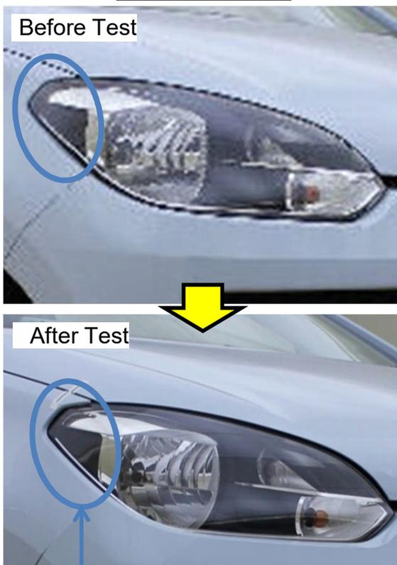
Due to the structure that helps prevent the headlight from interfering with the fender, damage to the fender is less likely to occur in a collision.
