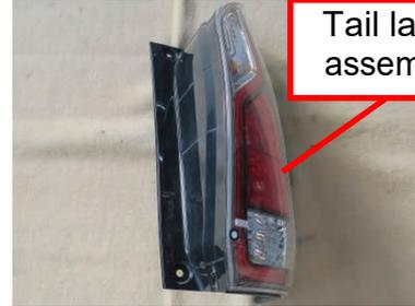
As the tail garnish was not supplied individually, the tail lamp assembly was replaced.
