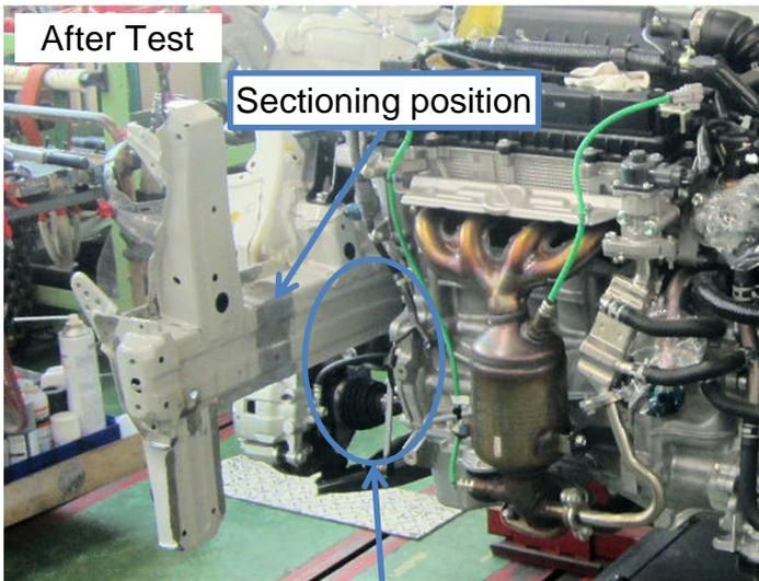
Only the auxiliary equipment had to be removed for sectioning.
