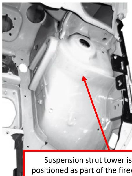
Suspension strut tower is positioned as part of the firewall plenum chamber and the front inner wing.
