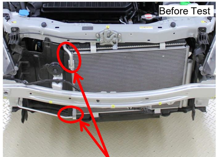
Two air conditioner condenser pipes are installed very close to the bumper
