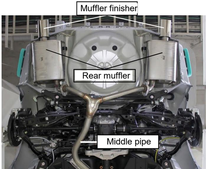
Middle pipe, rear muffler, and muffler finisher are supplied individually.
