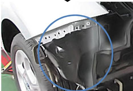
Only the lower section of the rear quarter panel was replaced.
