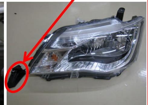
The bumper cover is attached to the headlight. Damage to the headlight is likely to occur.
