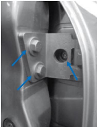
Good accessibility for panel beating operations. The side impact protection bar is mounted by bolts, so it is possible to remove it to facilitate access.
