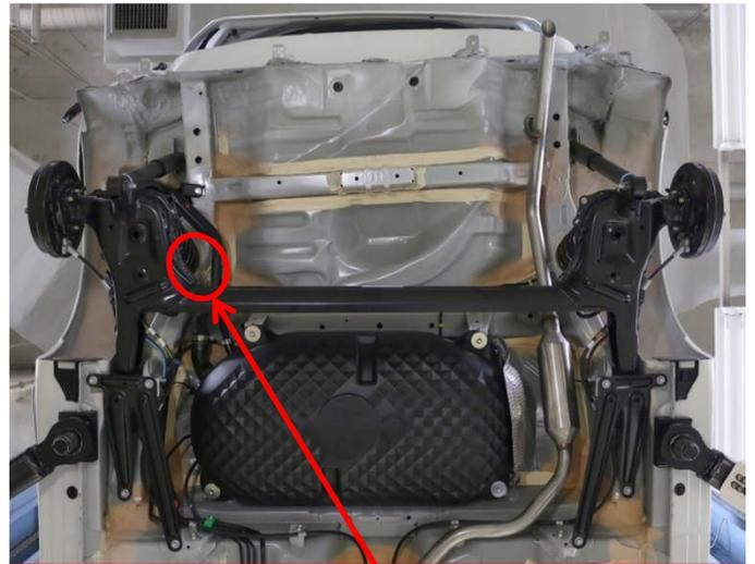
Rear side member extension was installed, but the damage spread to the side member.
