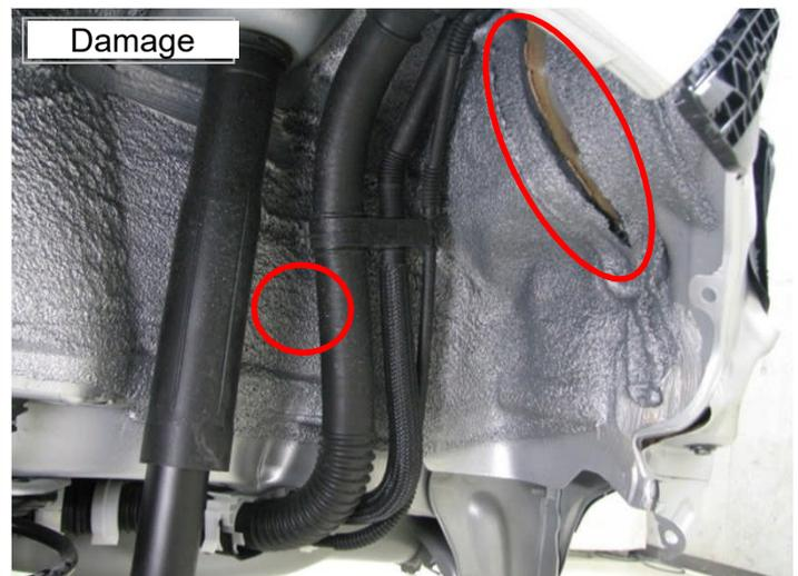
The rear side member and wheel housing were damaged and needed to be repaired.
