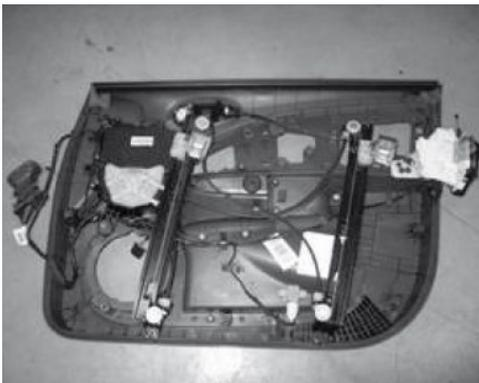
Most of the door mechanisms are fixed directly into its trim, which will facilitate repair and replacement operations.
