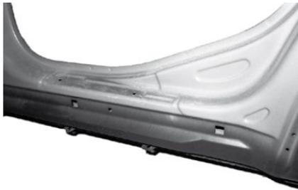
Sill cover panel runs from edge to edge over the reinforcement around the 'B' Post and rear reinforcement.
