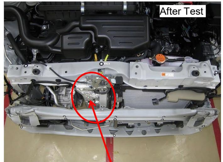
The exhaust manifold converter was pushed and damaged by the hood lock support.
