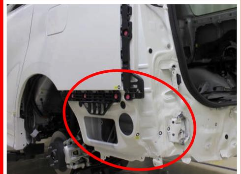
Although only the lower section of the rear quarter panel was damaged, the rear quarter panel assembly had to be replaced as sectioning was not an option.
