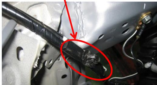
The harness clip on the side of the side member was damaged.
