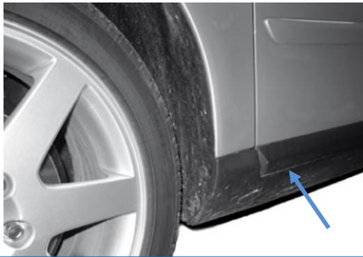
Sill cover panel runs from front edge to rear edge, over the reinforcement and around the 'B' Post and rear reinforcement. Sill shape is given by fitting a plastic cover.
