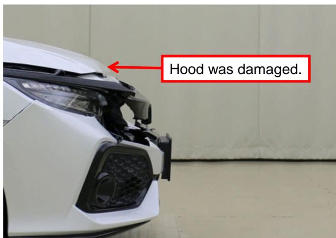
The hood was damaged because the front end of the bumper was lower than the barrier back stop.
