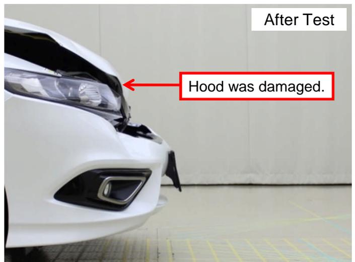
The hood was damaged because the distance from the front end of the bumper to the front end of the hood was shorter than the maximum collision penetration depth.
