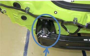
Crush box did not fall over, but was crushed.
