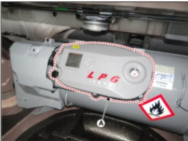
4. Fully close multi valve (A) to shut off the gas supply line.
