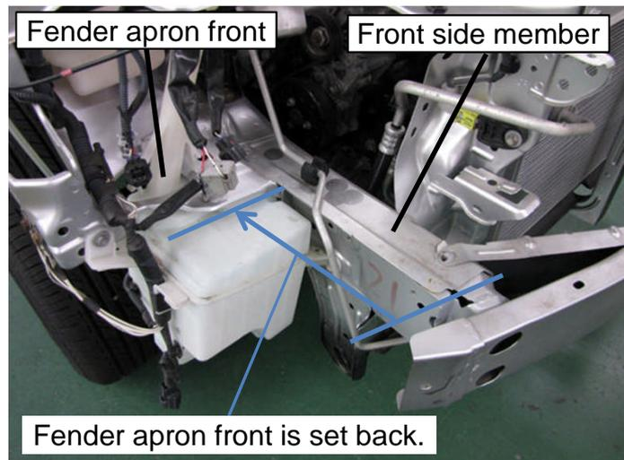
Example of a structure where the fender apron front is set back from the side member.
