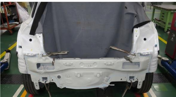
The adjacent panels did not have to be removed to replace the rear panel because the rear panel was installed in the outermost position.
