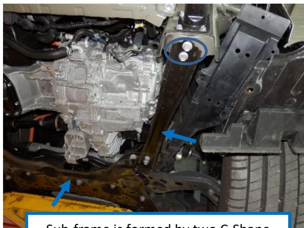
Sub-frame is formed by two C-Shape single parts, fitted via bolts.
