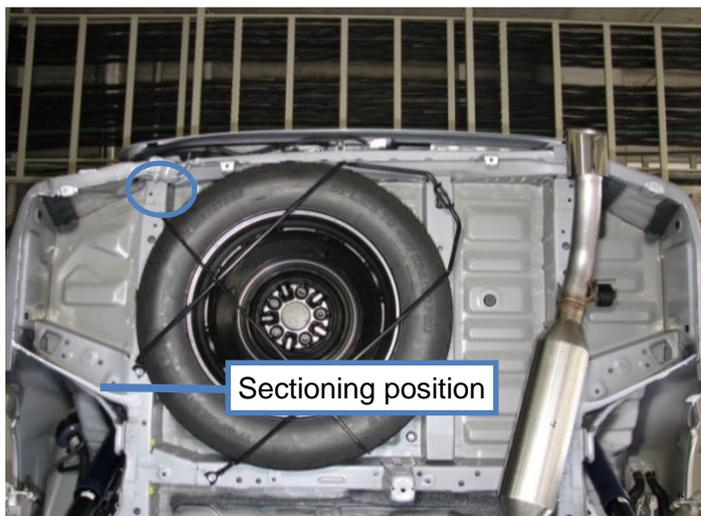
Damage ended aft of the sectioning position of the rear side member.
