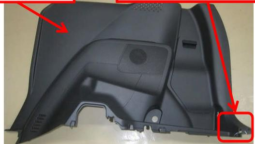
The quarter trim was part of the integral structure, so the entire assembly was replaced.
