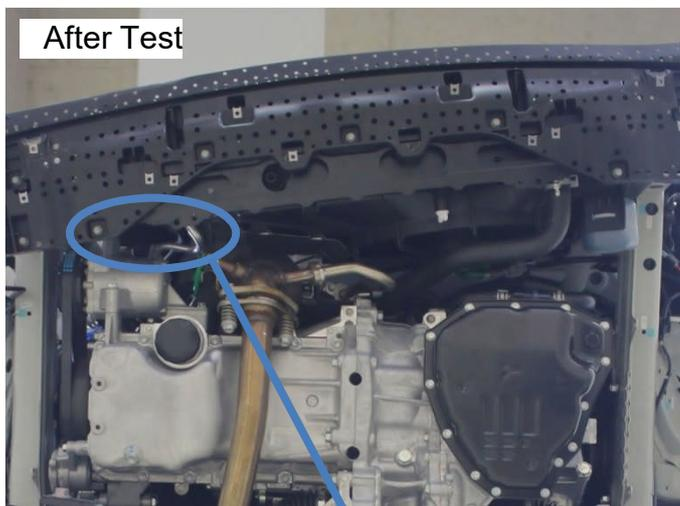
Neither the fan shroud or air conditioner condenser pipe was damaged.
