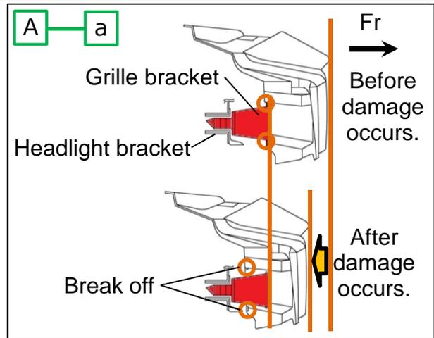
Example of a structure where the mating section of the radiator grille and headlight break off to prevent damage from spreading to the headlight.
