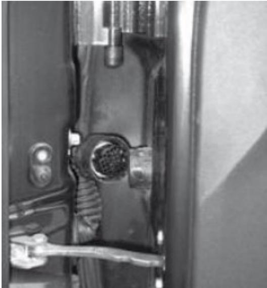
A central electrical multi-connector will make it easier to remove the door.
