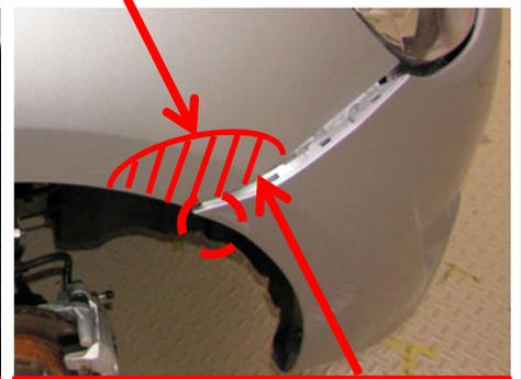
The ends are fastened with clips, so the fender would also be damaged.
