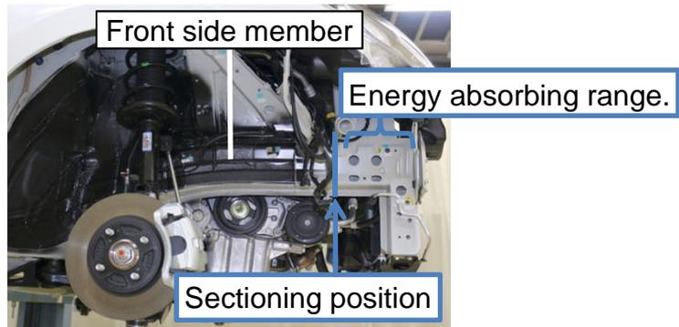
Example of a structure where damage ends before the sectioning position
