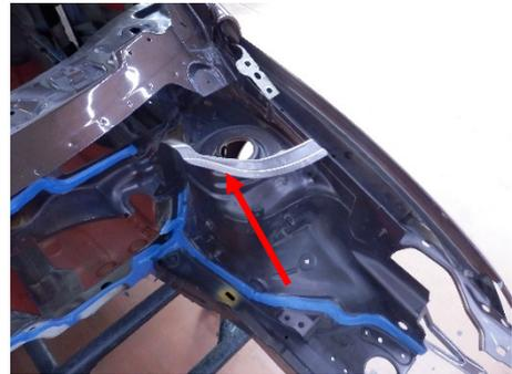
Disassembly of strut tower could be difficult due to the accessibility
