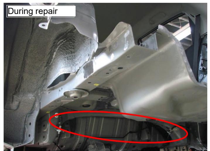
Removal of the fuel tank was necessary as the fuel neck is part of the fuel tank.
