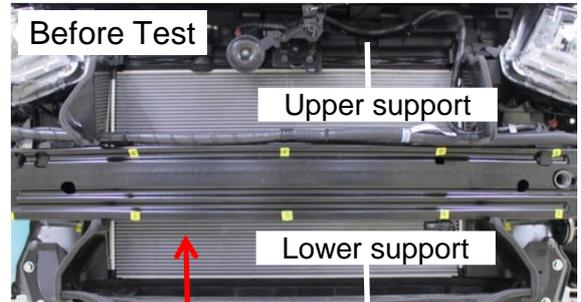
Condensers are installed on the upper and lower supports and damage is likely to spread from the bumper reinforcement and crush box.
