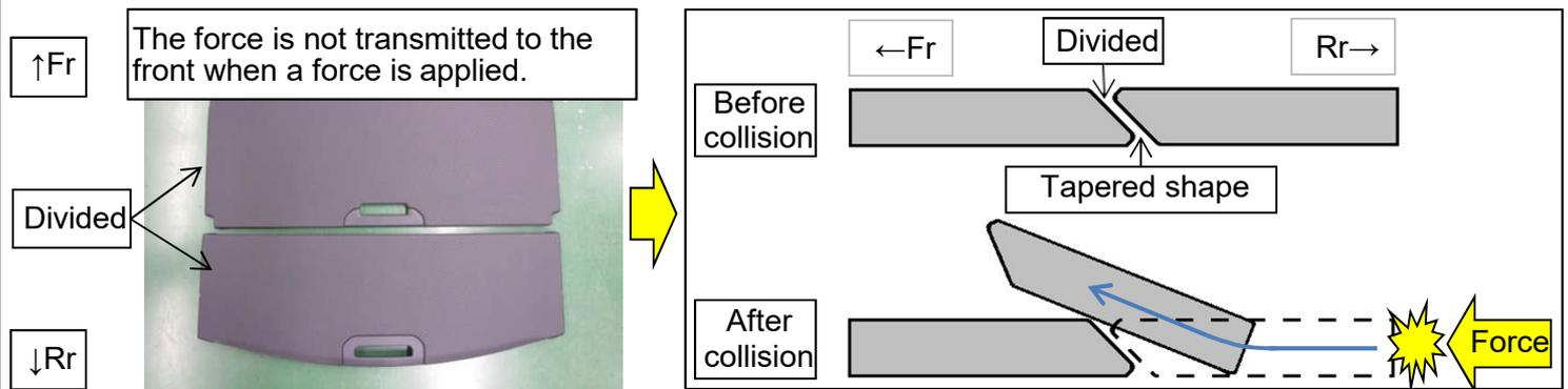
Example of a structure where the floor board trim is divided into front and rear sections so that applied force is not easily transmitted at the mating section.
