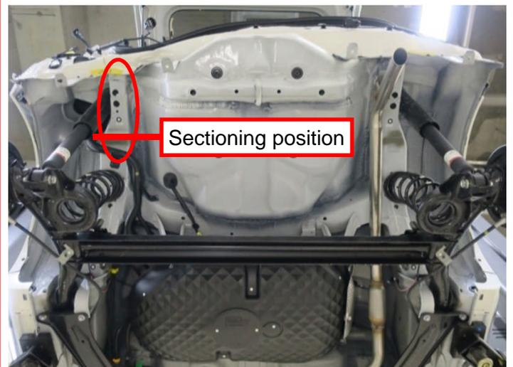
Damage spread past the sectioning position of the rear side member.
