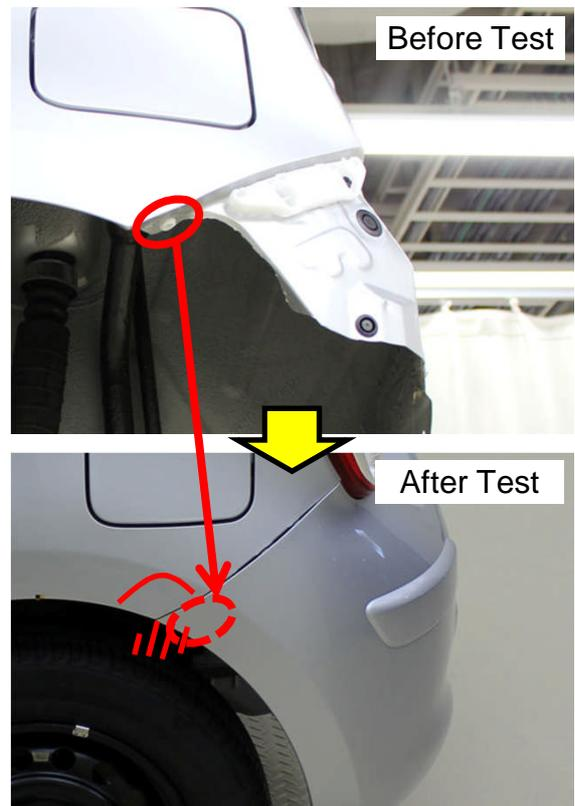
The ends were fastened with screws, which caused damage to the rear fender as well.
