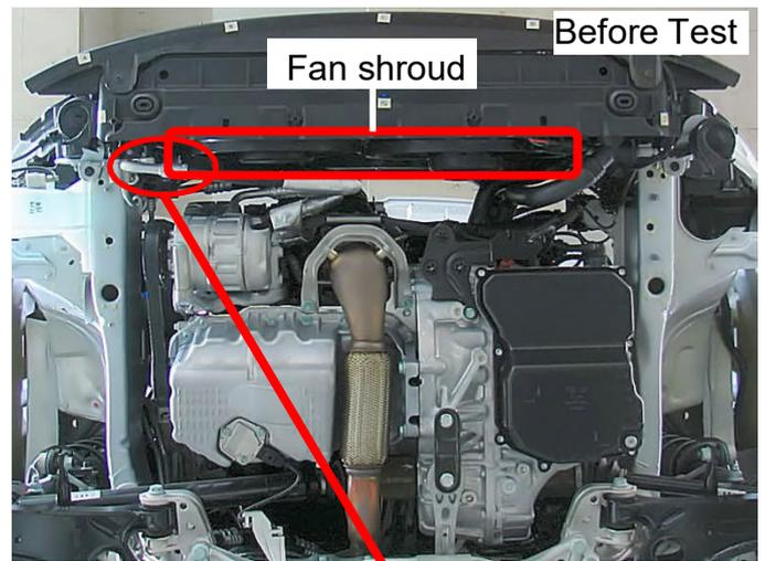
The clearance between the fan shroud and the air conditioner condenser pipe is not enough.
