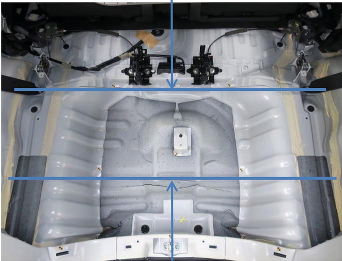
Sectioning position for when the damaged area is small.
