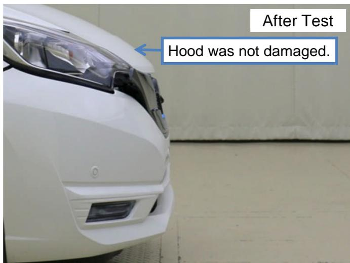
The hood was not damaged because the distance from the front end of the bumper to the front end of the hood was longer than the maximum collision penetration depth.
