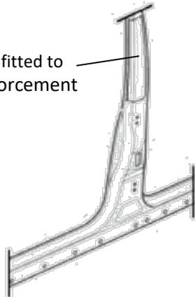
'B' Post with a UHSS reinforcement can be sectioned.
