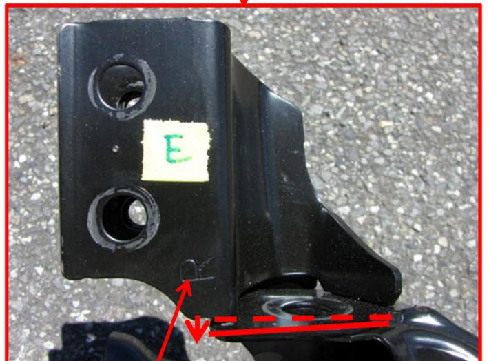
Suspension member mount is bent and damaged.
