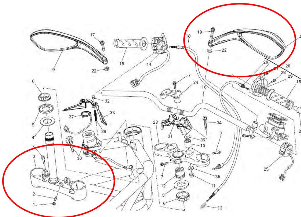
A3.20 The lower fork shank and frame should be reinforced in order that the frame is not deformed and the handlebar does not touch the fuel tank in a stationary fall.
