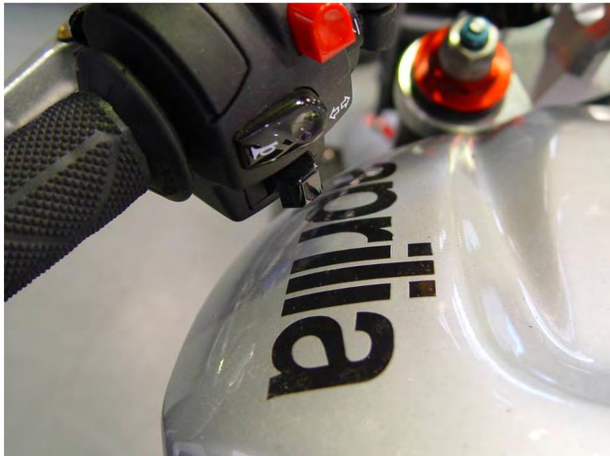
A3.4 Handlebar switches should have sufficient clearance from the fuel tank at full lock to ensure that fuel tank damage is avoided in a stationary fall.
