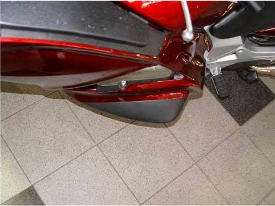
A3.13 Side facing bumper beams are an unobtrusive means to support a motorcycle when it falls over.
