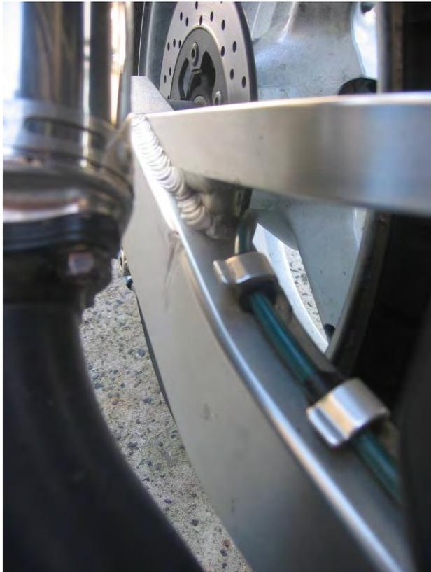
A3.8 The mufflers/silencers should not contact the rear suspension components, or crease the aluminium swingarm.
