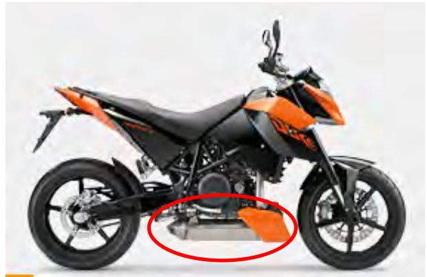
A3.19 Mufflers/silencers can be positioned under the seat or under the engine without protruding to the sides.
