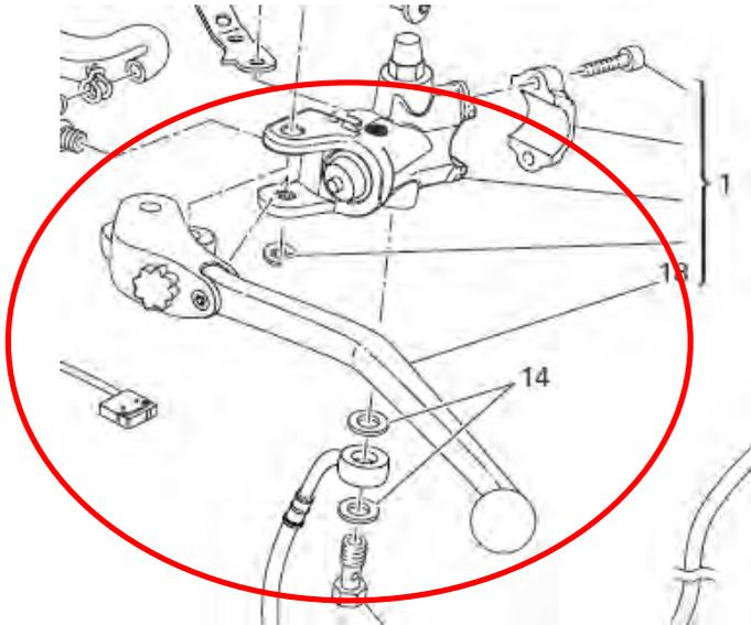
A3.18 Hand levers can pivot vertically to avoid snapping.
