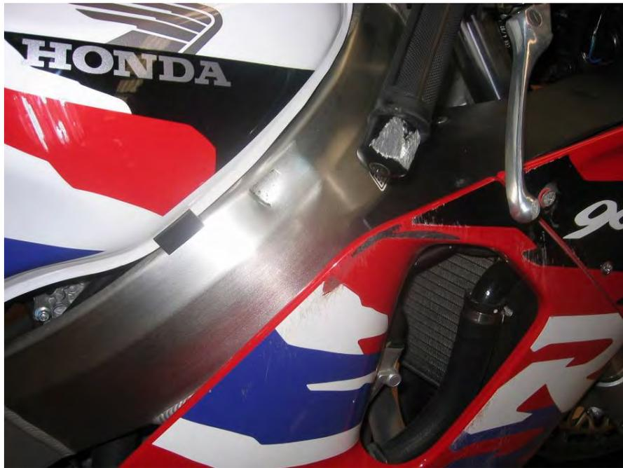
A3.3 The handlebar should not damage the fuel tank or the frame in a stationary fall.
