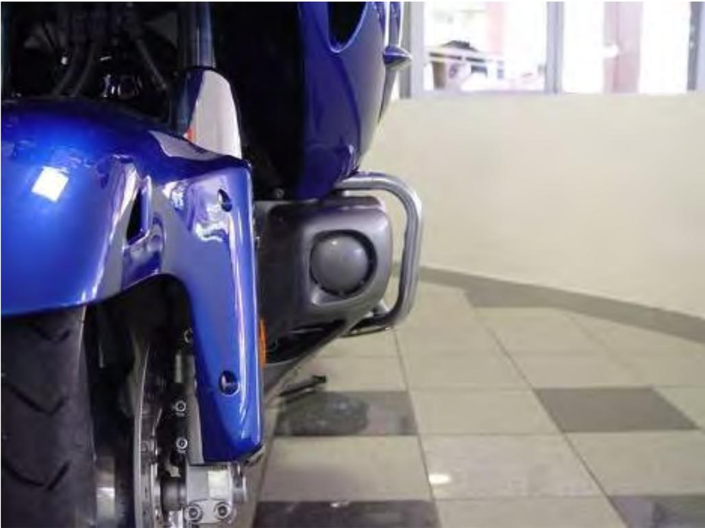
A3.13 Steel crash bars can be fitted unobtrusively.
