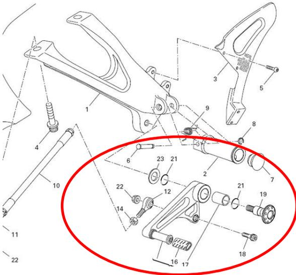
A3.17 Rubber on the inside of the lever could help to avoid frame damage. Gear and rear brake lever tips should hinge to the rear to avoid snapping off.
