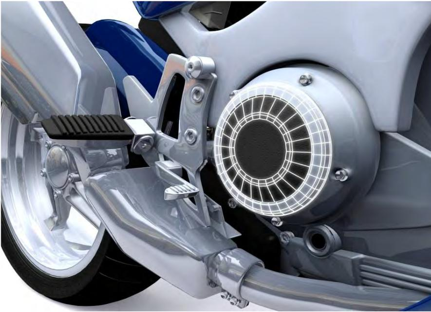
A1.8. Replaceable external clutch cover saves damage to engine, frame and ancillary components. Foot brake and gear levers are positioned so that frame damage is avoided. Springloaded levers return to position, rather than snapping off.
