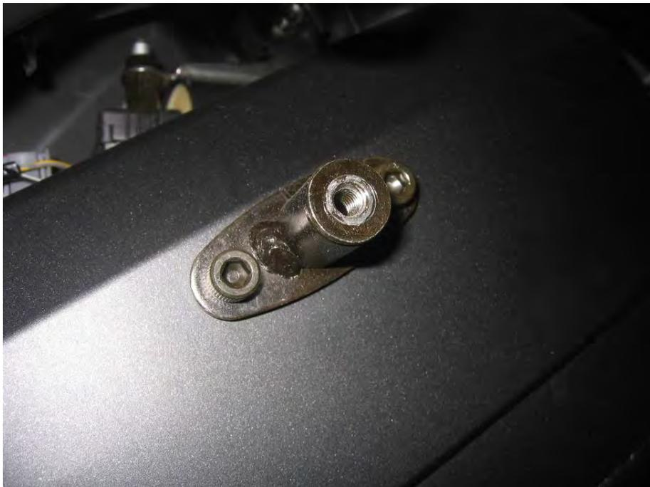
A3.6 Steel frame brackets should not be attached with steel bolts to an aluminium frames via aluminium threads.
