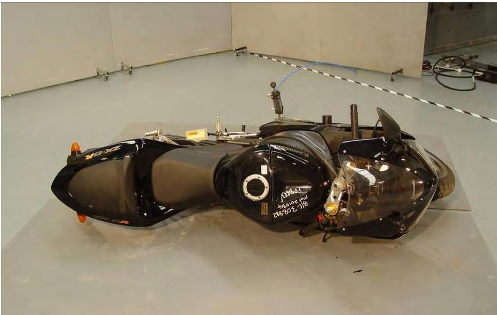
A2.4 The motorcycle is allowed to fall freely from the vertical position starting at close to zero velocity and falling over only under the influence of gravity.
