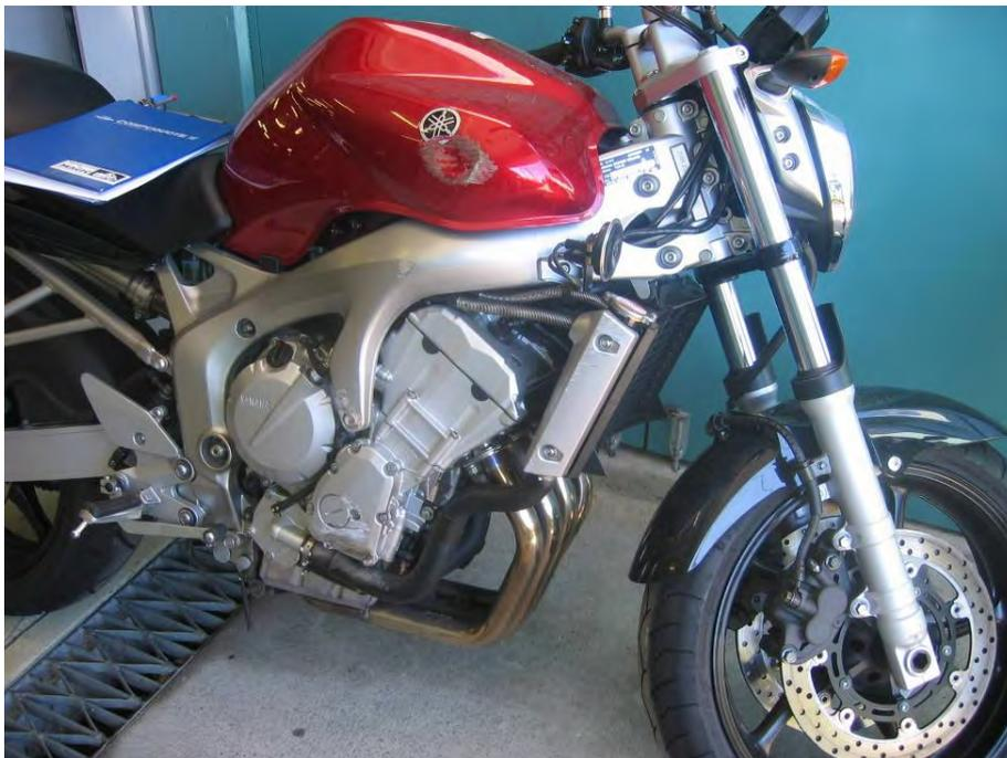
A3.2 The first points of contact in this stationary fall were the frame and fuel tank. The motorcycle was a total loss.
