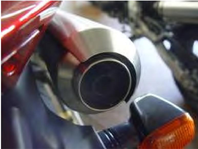
A3.7 Detachable heat shields should be used to prevent cosmetic damage to expensive exhaust mufflers/silencers.
