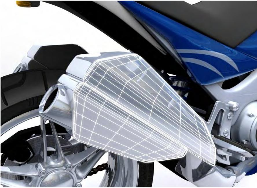
A1.14 Heat shield protects expensive muffler/silencer
