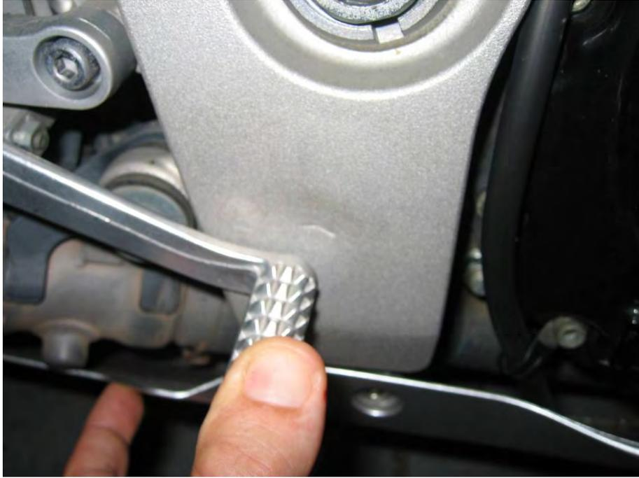
A3.5 Foot operated gear and brake levers should not damage the frame in a stationary fall.
