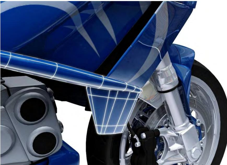
A1.9 Replaceable low-cost cover, supported by an internally reinforced steel bar, provides crash energy absorption and protects body side panels.
