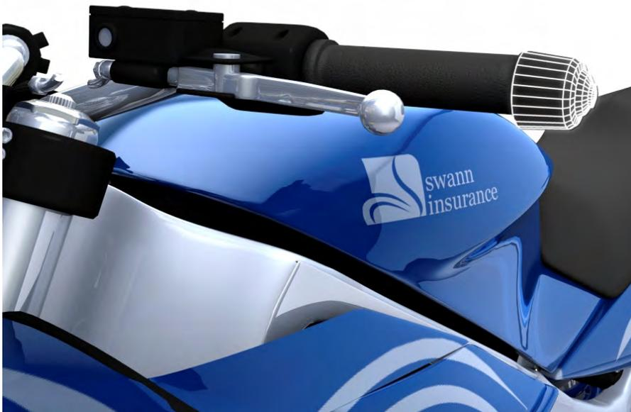
A1.13 Handlebar end cap absorbs impact energy. Handlebar lever pivots rather than snapping off.
