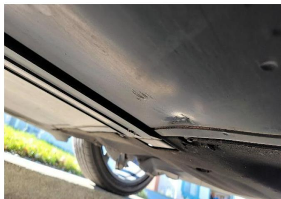
Figure 2 – HV Battery Minor Underbody Damage
