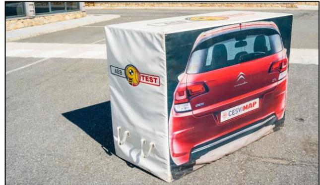
Figure 2 – CESVIMAP vehicle target
