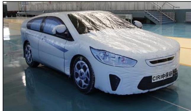
Figure 4 – CIRI inflatable vehicle target
