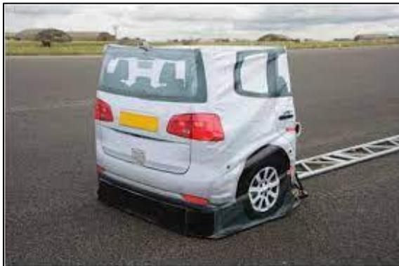
Figure 3 – Euro NCAP Vehicle Target (EVT)
