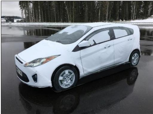
Figure 1 – Thatcham Research / AZT/IIHS Global Vehicle Target (GVT)
