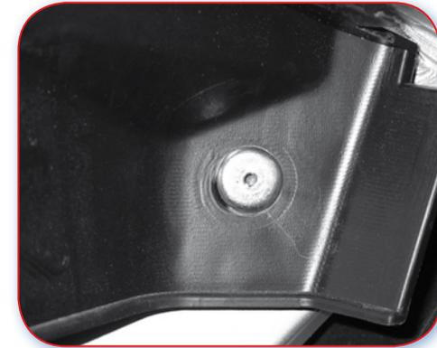
Poor Example. Plastic element fixed with rivets. Removal of the rivets could damage it.
