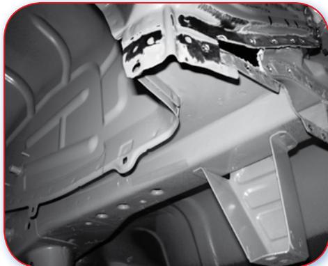
20.3.F There is enough space on the leg to deform and enough space between the leg and wheel arch to remove the leg.
