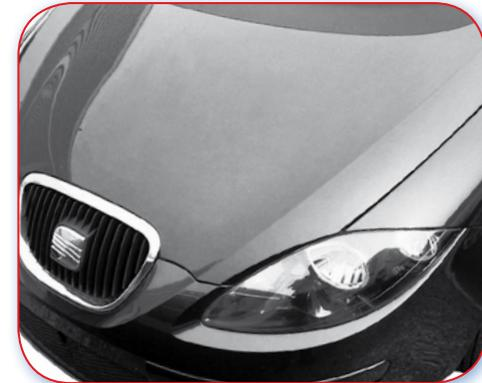
8.1.B Good example. Front edge of bonnet set back. Side edges protected by side panel.
