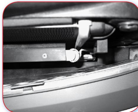
2.2.A Poor example. Not having enough distance between reinforcement and cooling pack - will cause damage to adjacent parts on impact.
