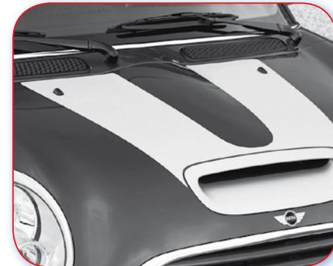
D.5.1 Poor example. A bonnet showing different colours on one panel.
