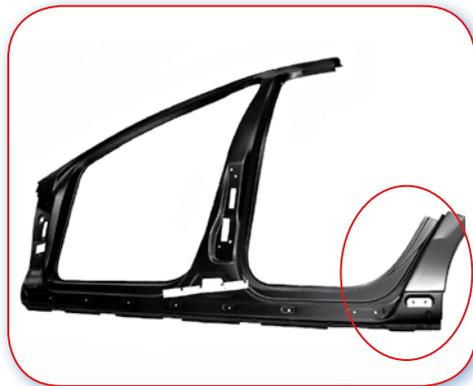
16.1.G Poor example. Service parts supplied as a side panel segment but having a joint at one of the most vulnerable and most frequently damaged parts like the dog leg.
