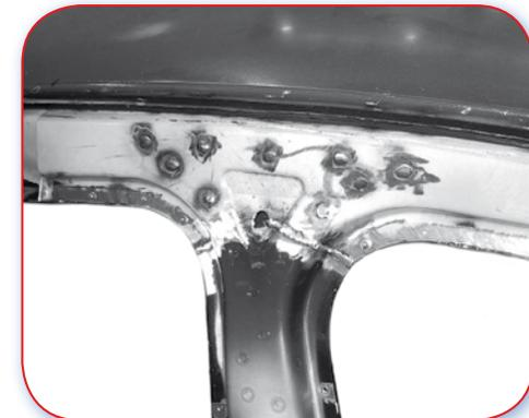
13.2.B Poor example. Damage must be avoided to the reinforcement due to limited space between the outer panel and reinforcements.
