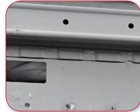
B.2.1 Poor example. Locations for new spot welds limited, due to shape of flange.
