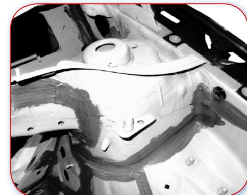
5.2.B Poor example. Suspension strut tower is positioned as part of the firewall plenum chamber.
