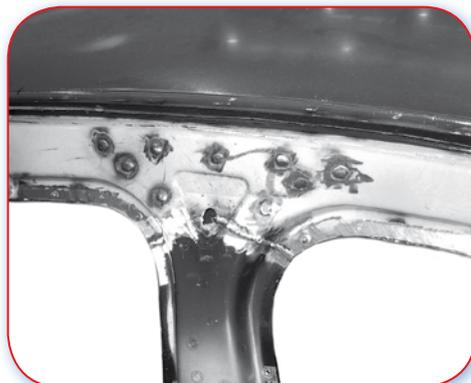
13.0.C 'B' Post has to be sectioned and roof rail has to be opened to allow the reinforcement to be fed between the panels, avoiding damage to the reinforcement due to space restrictions.
