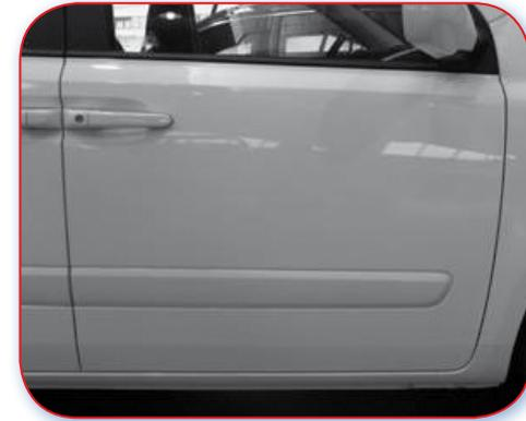
Poor Example. A moulding that does not cover the whole width of the doorskin does not allow painting of only part of the door.
