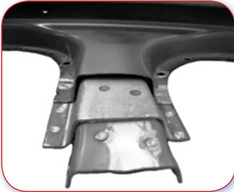
A.1.1 Poor example. Subsequent panels can be damaged during sectioning.
