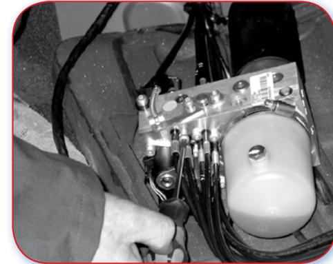
15.3.A Poor example. Hydraulic system to be drained before separation of the system from the folding roof.
