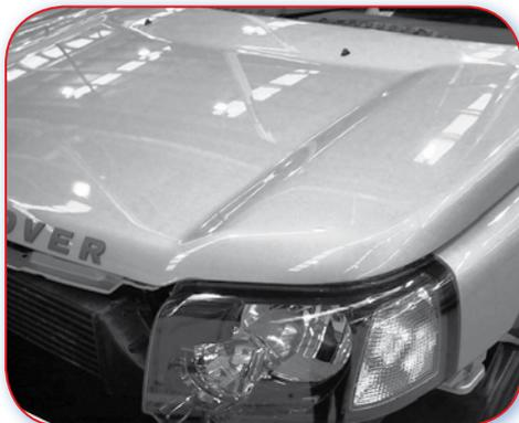
8.1.C Poor example. Wrap around bonnet which results in more exposure to damage.
