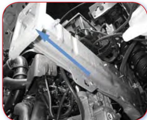
Poor Example. Front chassis leg without a central data point, does not have a suitable reference to control pulling operations.
