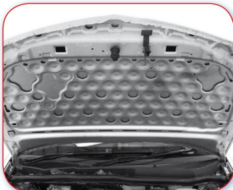
8.0.C Double skinned bonnet without reinforcing frame, compliant with the new pedestrian legislation. More difficult to repair, due to limited access to both panels.
