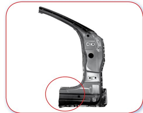
16.1.J Poor example. Service parts supplied in separate units need joining up when fitting, unless the part covers the damaged area.
