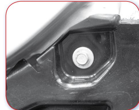
Good Example. Plastic element fixed with screws. Removing the screws is easy and causes no additional problems.
