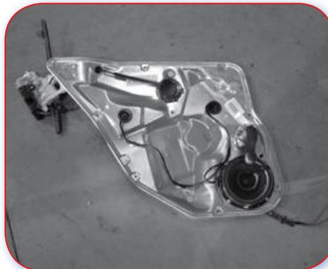
Good Example. The door has a screwed central frame, on which the various door mechanisms are fixed. This will allow the removal of the entire set, saving labour times.
