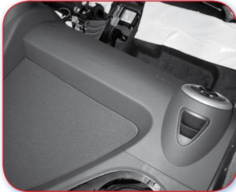
C.13.1 Good example. Facia can be partly removed after being damaged by deployment of airbag.
