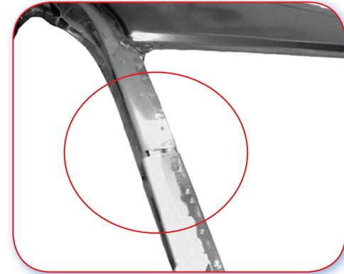
12.0.C Good example. 'A' Post reinforcement is sectionable at natural joint in upper part, avoiding complete removal.
