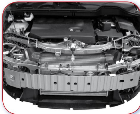
7.2.I Good example. Front panel bolted on.
