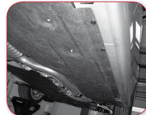
Poor Example. Covers under the vehicle will hinder the diagnosis and measurement of damage, as well as anchoring to the jig.
