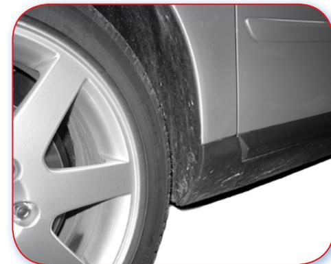
13.5.D Good examples. Sill cover panel runs from front edge to rear edge, over the reinforcement and around the 'B' Post and rear reinforcement. Sill shape is given by fitting a plastic cover.
