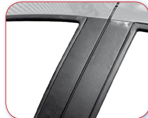
D.6.1 Poor example. Decal applied to door edges.
