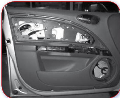
Good Example. A door trim with separate access covers will facilitate the disassembly and adjustment of door mechanisms without the need to remove trim.
