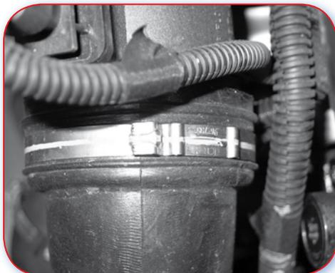
Poor Example. Conventional joints are difficult to remove, especially when access to the clip is restricted.
