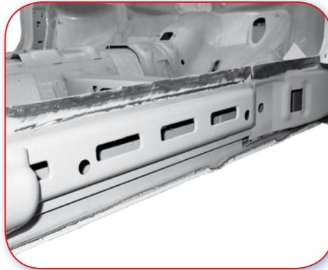
13.5.C Good example. Sill reinforcement is made of separate parts and can be repaired by partially removing the sill reinforcement.
