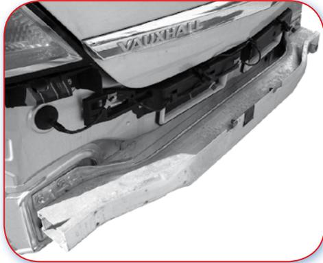
22.0.C Slight deformation of the beams.
