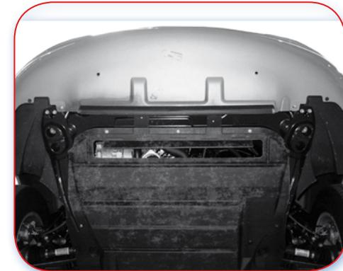
11.3.A Good example. Under tray covering engine bay, fixed with hexagonal head screws, not breakable clips or staples.
