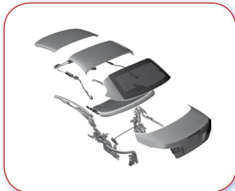
15.4.A Poor example. Folding roof assembly consisting of more than three panels.
