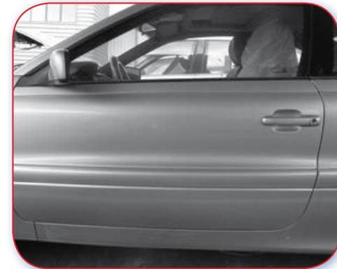
Good Example. A moulding across the whole door enables either the top or bottom of the door panel to be painted separately.
