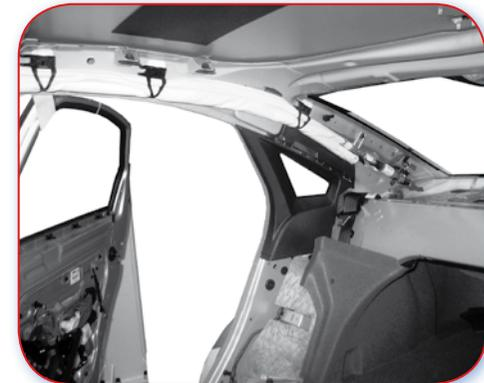
17.4.D Poor example. As the curtain airbag generator is fitted onto the rear roof joint, removal is required during repair.
