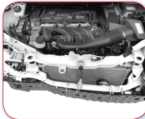
7.2.J Good example. Bonnet landing panel set back from the front bracket, avoiding subsequent damage.
