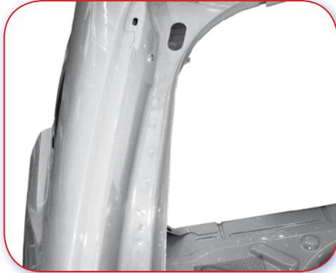
17.1.B Good example. Drain channel made out of one piece, joining outer and inner panel.
