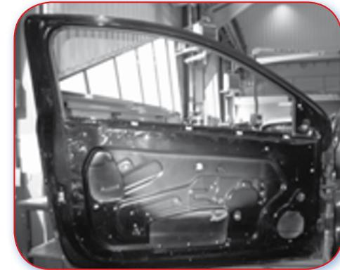
Poor Example. The limited access through holes in the door frame makes repair difficult.
