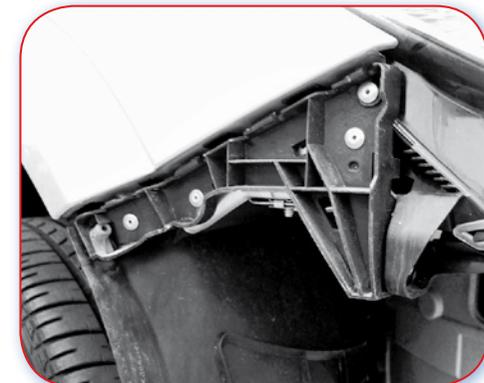
1.1.D Poor example. Bracket is supporting the panel and bumper independently. Fastener for the panel is covered by the bracket.
