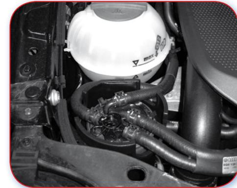
C.4.1 Poor example. Expensive auxiliary units positioned in vulnerable areas.
