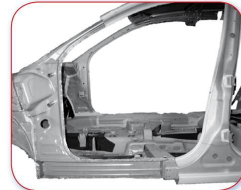
13.1.C Good example. 'A' Post cover and reinforcement where it joins the sill which are sectionable, making removal of the 'A' Post reinforcement easier and allowing for sectioning of the sill.
