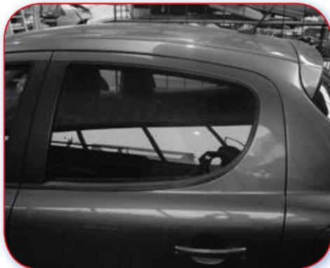
Poor Example. A doorskin with window frame will be difficult to replace.
