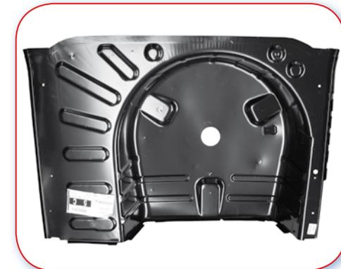
19.0.D Poor example. Boot floor area in BIW without reinforced plastic infill and service repair part.
