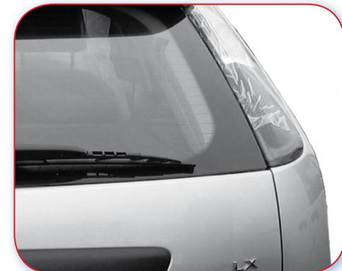
C.6.1 Good example. A light cluster fitted in a higher position avoids damage on impact.
