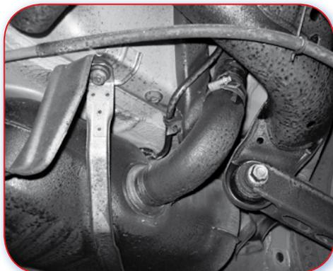
C.2.1 Fuel filler neck and fuel tank joint with removable elbow, allowing it to be separated.
