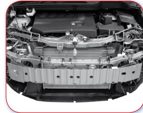
2.1.A Good example. Good distance between reinforcement and cooling pack. Good reinforcement height and no parts clip onto it.
