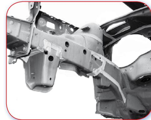
9.3.A Good example. These pictures show chassis legs with natural joints near the firewall for complete replacement.
