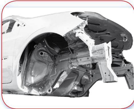
D.1.1 Poor example. Body showing different finishes.
