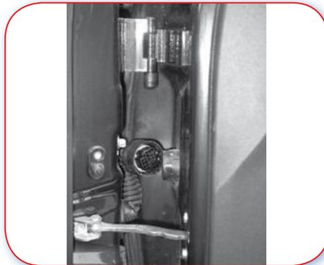
Good Example. A central electrical multi-connector will make it easier to remove the door.
