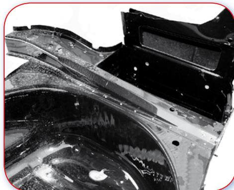
20.3.B Poor example. The chassis leg is part of the boot floor and therefore difficult to take apart.
