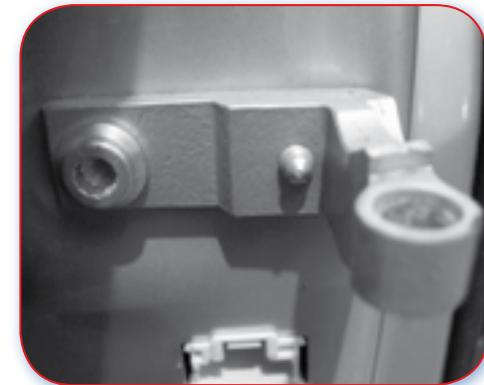
Poor Example. The limited access through holes in the door frame causes problems in repair.
