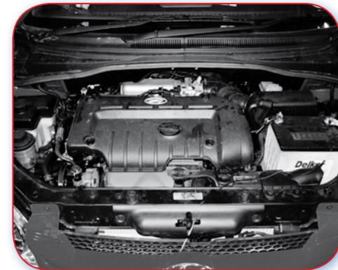
7.2.H Good example. The front panel comprises a landing panel but no lower parts. Costly parts set back enough to reduce damage.
