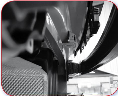
Good Example. Rear centre panel with the flange pointing downwards facilitates drilling and welding operations.
