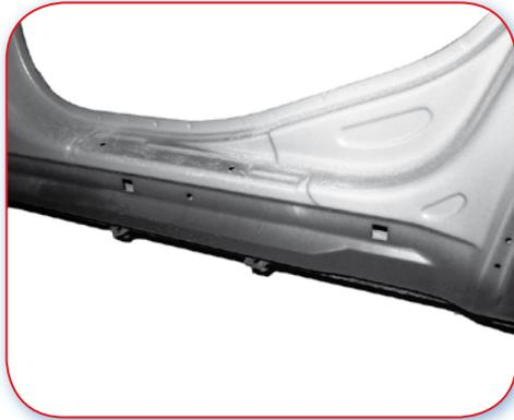
13.4.B Good example. Sill cover panel runs from edge to edge over the reinforcement around the 'B' Post and rear reinforcement.
