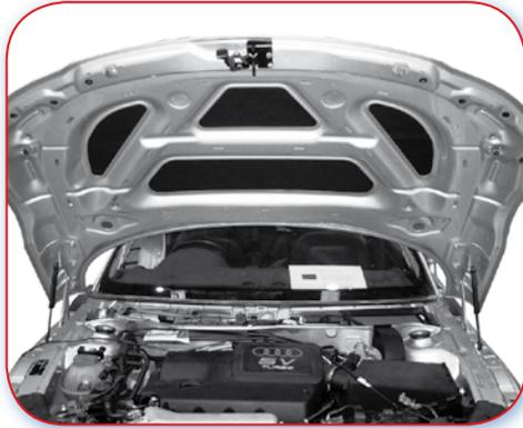
8.0.A Single skinned bonnet with reinforcing sub-frame, easier to repair as both panels are accessible.
