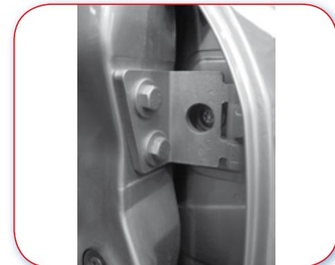
Good Example. Good accessibility for panel beating operations. The side impact protection bar is mounted by bolts, so it is possible to remove it to facilitate access.
