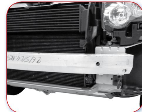
2.1.C Good example. Good reinforcement height. Good distance between bumper beam and cooling pack. Low pedestrian protection bar. No parts fixed to the bumper beam.
