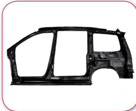
16.1.C Good example. Service parts supplied as a whole that can be cut where required to suit the damage to the vehicle. This avoids any mismatching joints.
