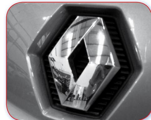
1.6.C Poor example. The badge fixed to the bumper panel and the fastener for the panel is covered by the bracket.
