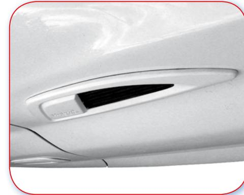
D.4.1 Poor example. A hard plastic insert is difficult to mask around, so it will require removal.
