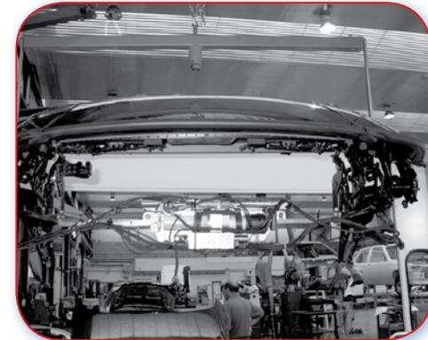
15.3.B Good example. The complete assembly, including electro hydraulic system, can be removed.
