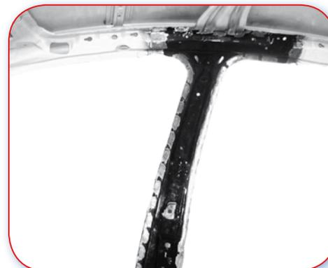
13.2.C 'B' Post cannot be sectioned so the roof rail has to be opened to allow the 'B' Post panel with its 'non-weldable' press hardened reinforcement, to be fitted onto the roof rail and sill.
