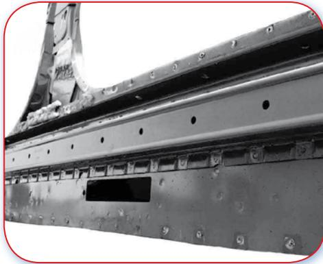
13.5.B Poor example. Sill reinforcement is a single piece and when damaged will require sill cover removal and sectioning.
