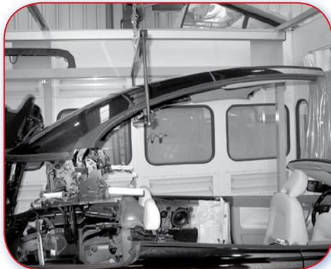
15.1.C Good example. The whole assembly is easily removed from the vehicle due to availability of moving space.
