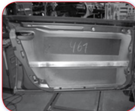
Good Example. Good accessibility for panel beating operations. The side impact protection bar is mounted by bolts, so it is possible to remove it to improve the accessibility.
