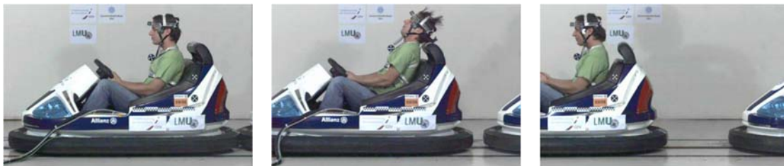
Fig. 15 Actual movement of head in a rear impact situation without head rest supporting the head (AZT Automotive GmbH)
