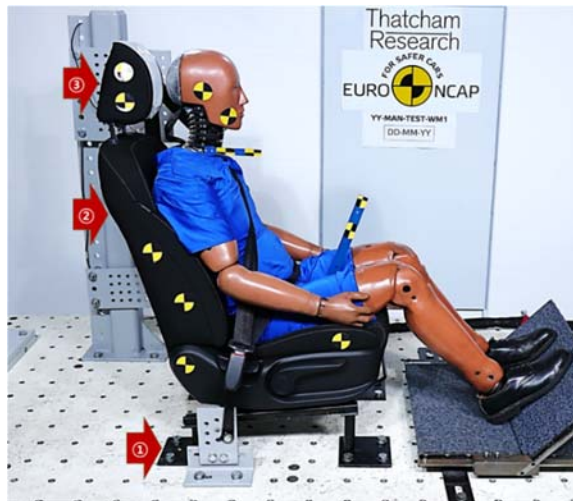
Fig. 13 Application of force to the occupant in the struck vehicle during rear-end collisions or in the striking vehicle during reverse collisions
