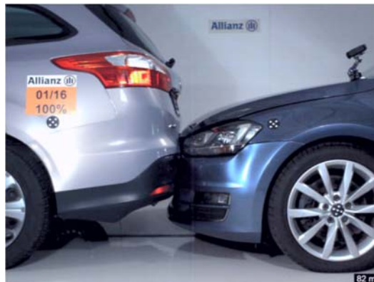
Fig. 4 Full overlap rear-end collision
