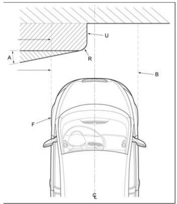
The height of the barrier shall exceed the height of the front of the test vehicle. The test vehicle shall be free of any propelling device at the point of impact.
