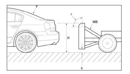
Key: MB = Mobile Barrier H = Barrier height (700mm+/-10 mm) h = Ground clearance (200 mm +/- 10 mm) F = Test vehicle R = Constant radius (150 mm) r = Constant radius (50 mm) U = 40% Overlap B = Vehicle width (rear)
