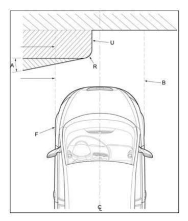
At the moment of impact the vehicle shall be free of the vehicle propulsion system.
