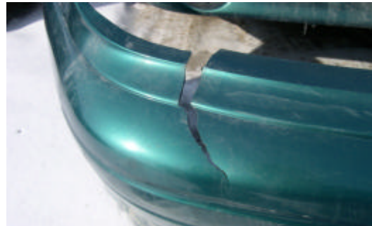
Two sided repairs for cuts or splits in the base material
