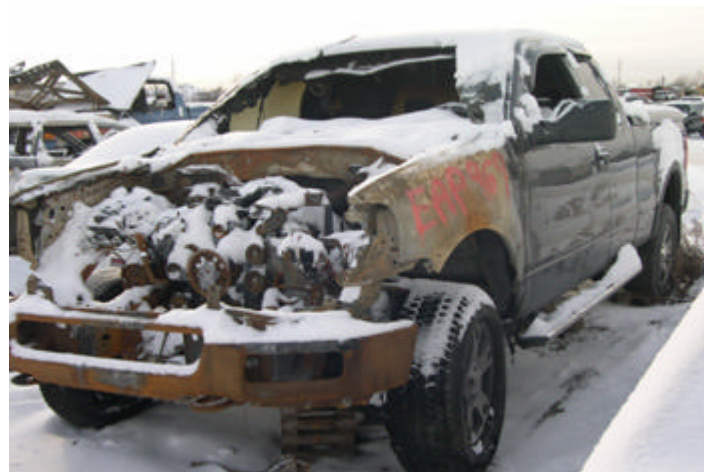
Figure 1—Fire consumed the engine compartment and interior cabin
