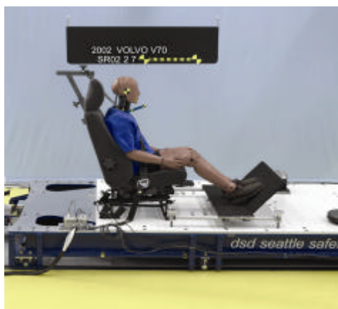
Dynamic tests are being conducted on a sled that reproduces a typical rear impact
