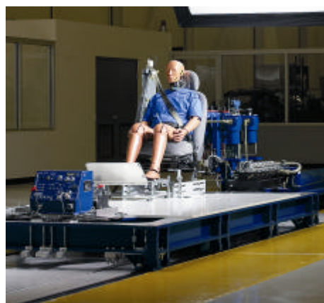
BioRID IIg has an articulated spine that bends in a human like manner
