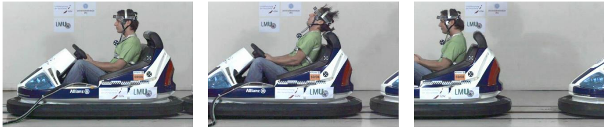
Fig. 12 Actual movement of head in a rear impact situation without head rest supporting the head (AZT Automotive GmbH)
