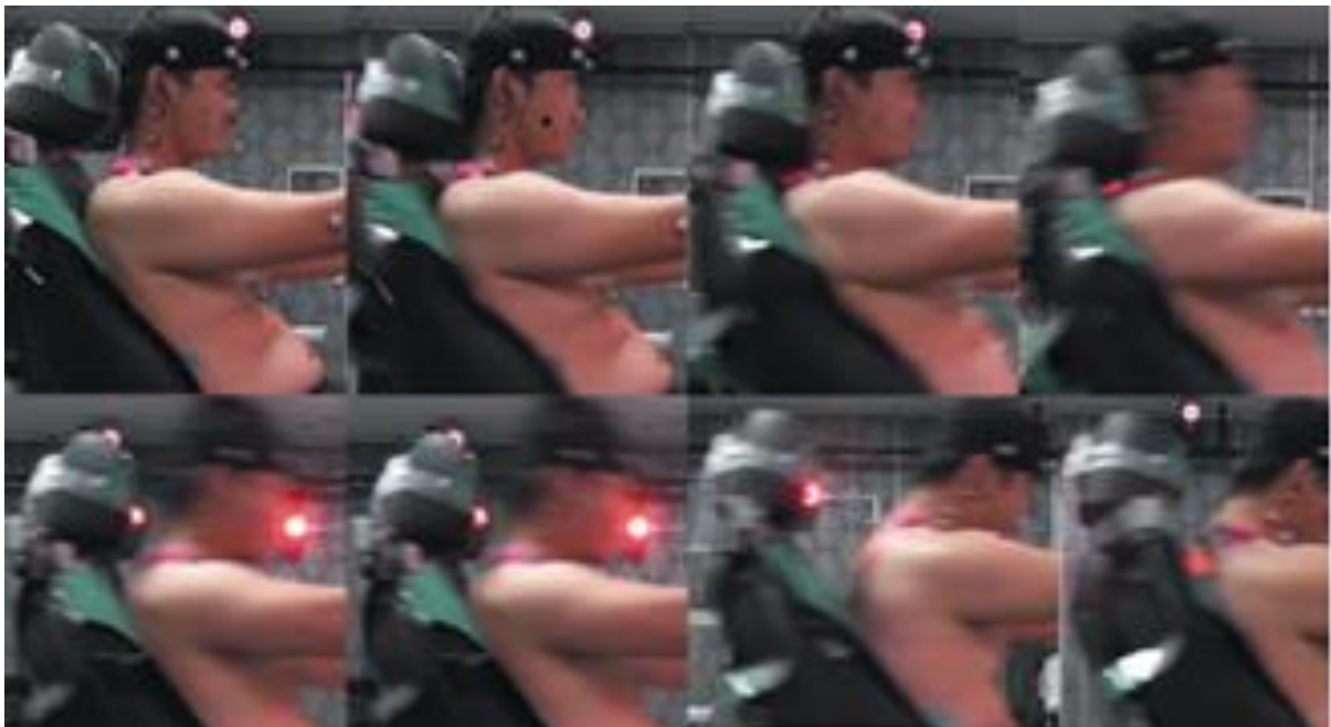
Fig. 32 Movement of a human volunteer at 7.9 km/h of \Delta V
