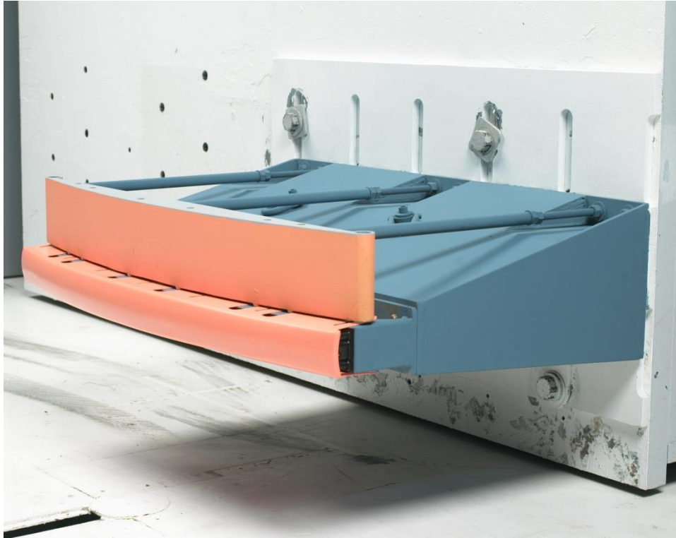
Figure 4: Complete Bumper Barrier with Backstop, Cover, and Energy Absorber
