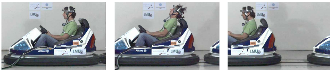
Fig. 13 Actual movement of head in a rear impact situation without head rest supporting the head (AZT Automotive GmbH)
