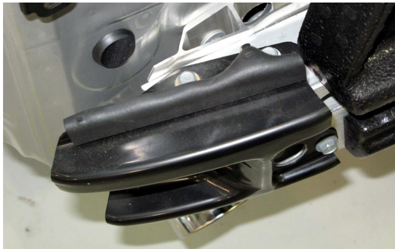
Figure 11. Example of bolt on extension
