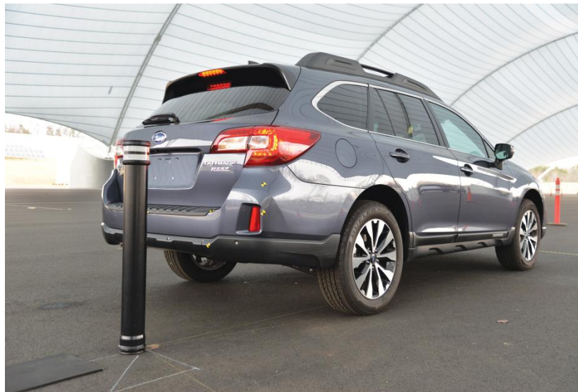
One of the tests in the new IIHS rear crash prevention assessment evaluates rear autobrake's ability to stop a reversing car from striking a pole.
