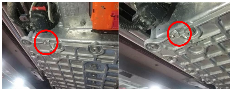
Figure 2. Ford Escape HEV high voltage battery damaged due to an underbody bump.
