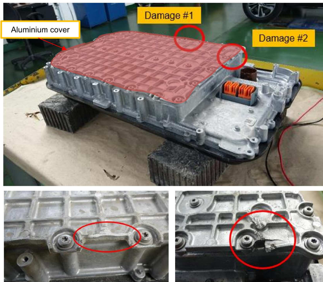
Figure 1. Damage in the battery: external visual inspection
