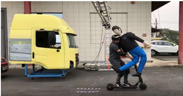
Dynamic braking test developed at 20 Km/h
