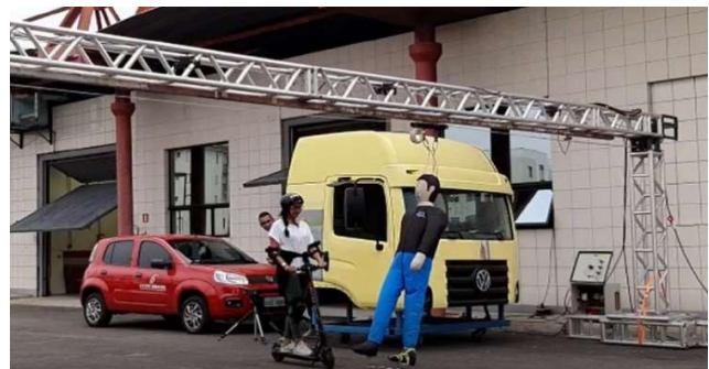
Dynamic braking test developed at 10 Km/h
