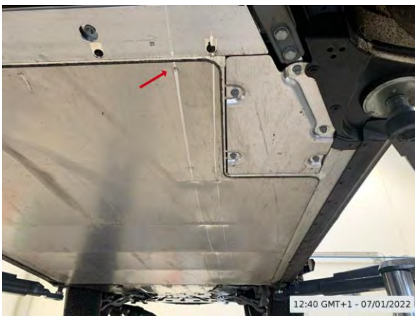
Typical example for damage to unprotected high voltage battery
