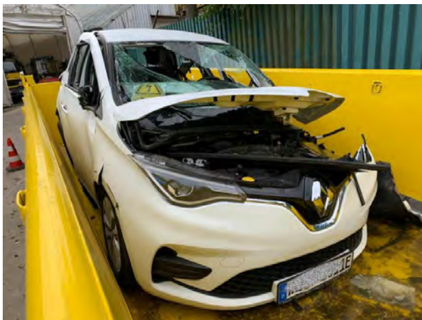
Example for quarantine handling of high voltage vehicle
