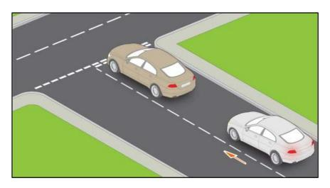
Figure 2 – Car-to-car front-to-rear collision test scenario
