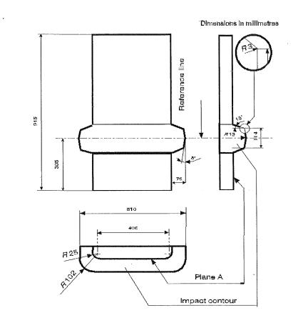
The impactor axis height is to be 445 mm from the ground surface, both for front devices and rear devices.
