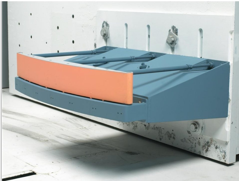
Figure 1: Steel Bumper Barrier with Backstop
