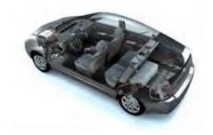
Toyota plans to add optional solar panels on the roof to Prius III, its next generation 'hybrid' in 2009, in order to power the vehicle's air conditioning whilst parked <sup>8</sup>. Combining a two high voltage electric motors, an 'Atkinson' cycle internal combustion engine (very low emission),
