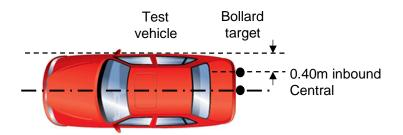
Figure 8 – Reversing car-to-bollard central and 0.40m inbound at impact position
