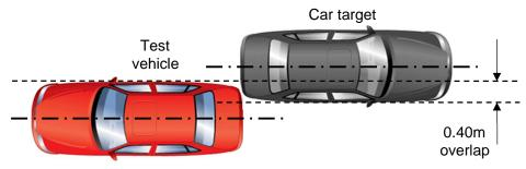
Figure 3 – Reversing car-to-car 0.40m overlap at impact position
