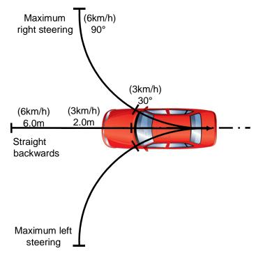
Figure 6 – Reversing car-to-car manoeuvres and ranges
