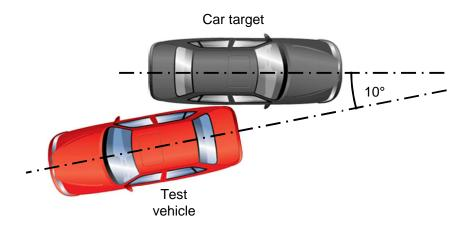
Figure 6 – Reversing car-to-car 10° side at impact position
