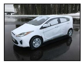
Figure 1 – Global Vehicle Target (GVT)
