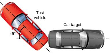
Figure 4 – Reversing car-to-car 45° centre at impact position
