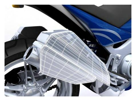
A1.14 Heat shield protects expensive muffler/silencer
