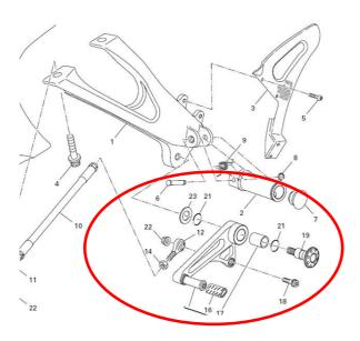
A3.17 Rubber on the inside of the lever could help to avoid frame damage. Gear and rear brake lever tips should hinge to the rear to avoid snapping off.
