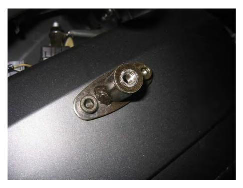
A3.6 Steel frame brackets should not be attached with steel bolts to an aluminium frames via aluminium threads.
