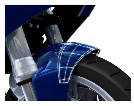
A1.11 Two-piece front mudguard detaches to reduce replacement cost.
