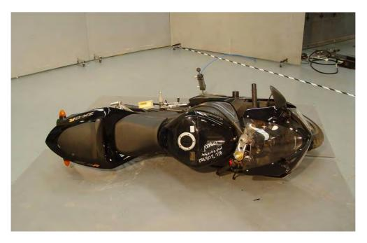
A2.4 The motorcycle is allowed to fall freely from the vertical position starting at close to zero velocity and falling over only under the influence of gravity.
