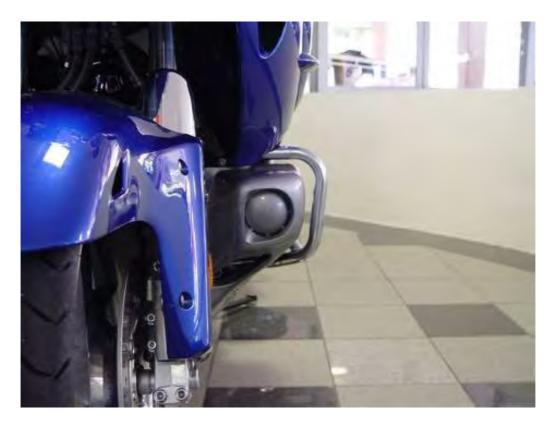
A3.13 Steel crash bars can be fitted unobtrusively.
