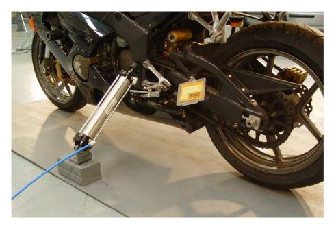
A2.1 The motorcycle is drained of fuel and positioned almost vertically on a hard horizontal surface. The preferred material is a fibre reinforced cement with a painted surface and a fine sand abrasive added. The front and rear wheels are placed in line and the transmission is placed in neutral.
