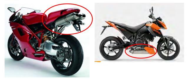
A3.19 Mufflers/silencers can be positioned under the seat or under the engine without protruding to the sides.
