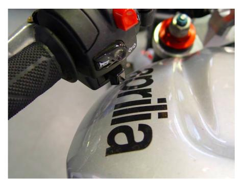
A3.4 Handlebar switches should have sufficient clearance from the fuel tank at full lock to ensure that fuel tank damage is avoided in a stationary fall.
