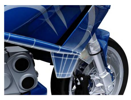
A1.9 Replaceable low-cost cover, supported by an internally reinforced steel bar, provides crash energy absorption and protects body side panels.
