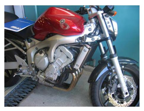
A3.2 The first points of contact in this stationary fall were the frame and fuel tank. The motorcycle was a total loss.
