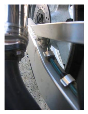
A3.8 The mufflers/silencers should not contact the rear suspension components, or crease the aluminium swingarm.
