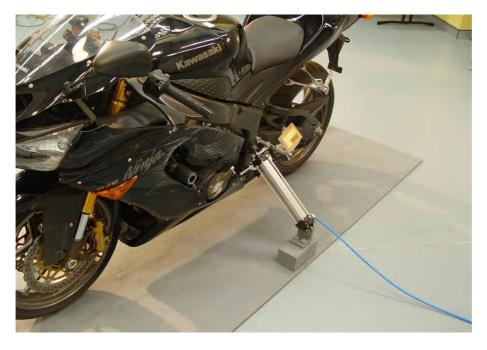
A2.2 The side and centre stands are folded up and the motorcycle is supported on the opposite side by a double acting air cylinder.
