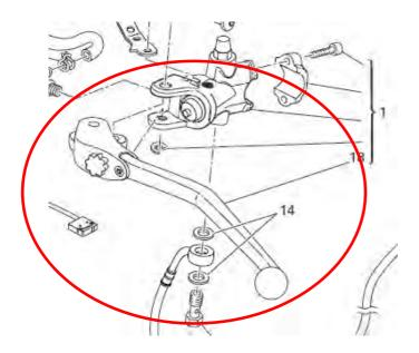
A3.18 Hand levers can pivot vertically to avoid snapping.
