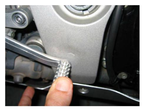
A3.5 Foot operated gear and brake levers should not damage the frame in a stationary fall.
