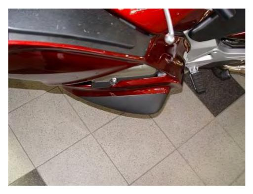
A3.13 Side facing bumper beams are an unobtrusive means to support a motorcycle when it falls over.
