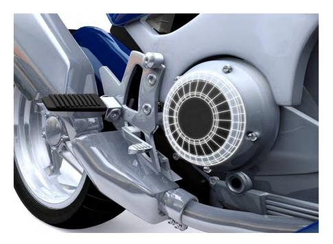
A1.8. Replaceable external clutch cover saves damage to engine, frame and anciliary components. Foot brake and gear levers are positioned so that frame damage is avoided. Springloaded levers return to position, rather than snapping off.
