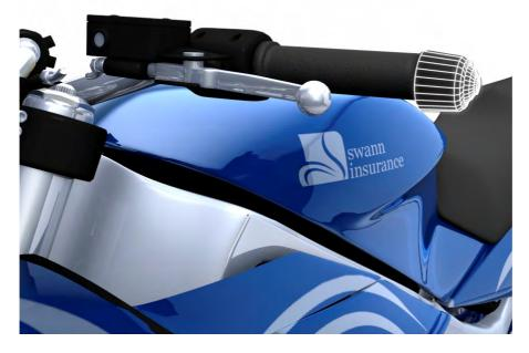
A1.13 Handlebar end cap absorbs impact energy. Handlebar lever pivots rather than snapping off.
