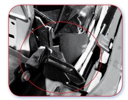
7.2.F Good example. This panel can be replaced easily. The cooling pack can move, but will not be damaged on impact.
