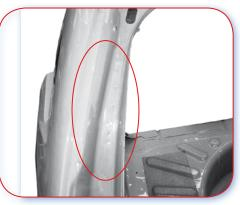
17.2.D Good example. The drain channel is made out of one piece, joining the outer and inner panel.
