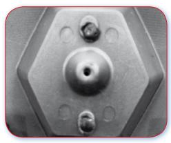
1.6.B Poor example. The badge fixed to the bumper panel and the fastener for the panel is covered by the bracket.
