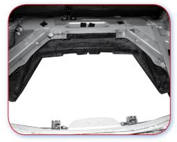
20.3.G Note 1. Good example. Ample access after plastic boot floor insert has been removed.
