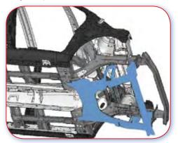
10.0.C Good example. Sub-frame as a two piece unit. Separable
