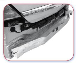
22.0.C Slight deformation of the beams.
