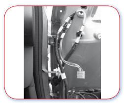
Poor Example. The door does not have a central electrical multi-connector, so it is necessary to remove the door trim and to disconnect the different electrical devices
