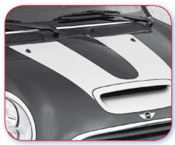
D.5.1 Poor example. A bonnet showing different colours on one panel.
