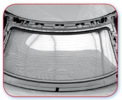
15.8.A Poor example. Glass panel bonded into complex shaped folding roof panel.
