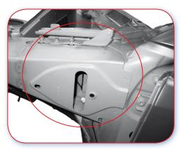
12.1.A Good example. Bridging plate creates a joint between 'A' Post and side panel reinforcement, easing removal of both panels.
