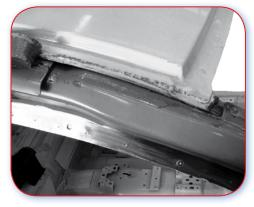
12.1.D Good example. Outer panel fitted over roof panel.
