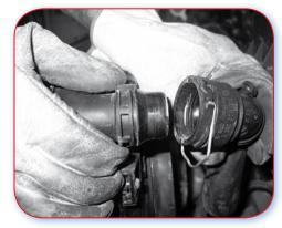
Good Example. Quick plug joints facilitate removal of the mechanical elements.
