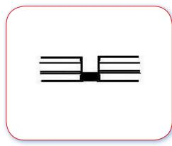
B.4.2 Step two: Spot weld removed to allow removal of outer panels.
