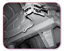
20.3.F There is enough space on the leg to deform and enough space between the leg and wheel arch to remove the leg.
