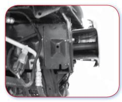
3.0.D Poor example. No crush can, so the chassis leg will be damaged on impact.
