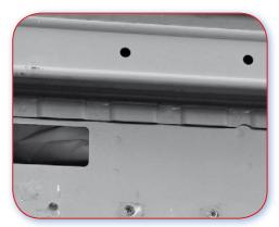
B.2.1 Poor example. Locations for new spot welds limited, due to shape of flange.
