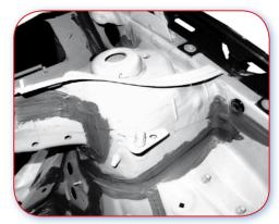
5.2.B Poor example. Suspension strut tower is positioned as part of the firewall plenum chamber.
