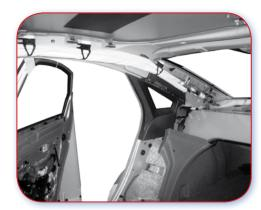
17.4.D Poor example. As the curtain airbag generator is fitted onto the rear roof joint, removal is required during repair.
