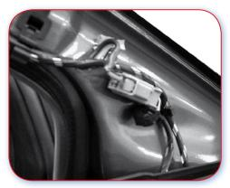
C.7.2 Poor example. Loom partly detachable. Use a larger multiplug or an additional plug, so both sets of wires can be detached.
