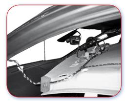
C.7.1 Poor example. Parts and looms that cannot be detached.
