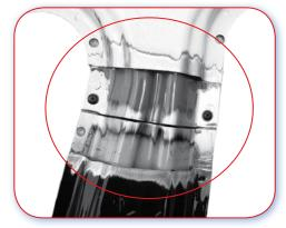
13.2.H 'B' Post can be sectioned through reinforcements and both outer and closing panel without having to cut into upper roof rail. Most reinforcements made from UHSS cannot be sectioned.
