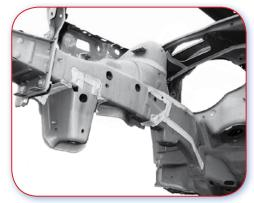
9.3.A Good example. These pictures show chassis legs with natural joints near the firewall for complete replacement.
