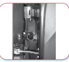
Good Example. A central electrical multi-connector will make it easier to remove the door.
