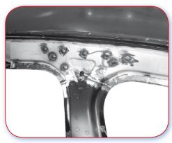
13.2.B Poor example. Damage must be avoided to the reinforcement due to limited space between the outer panel and reinforcements.
