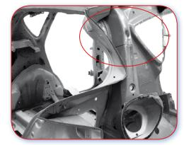
17.1.F Poor example. The reinforcement requires removal of the side panel before it can be replaced. The drain channel is made of separate parts, making alignment and positioning difficult.
