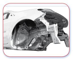
D.1.1 Poor example. Body showing different finishes.
