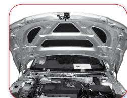
8.0.A Single skinned bonnet with reinforcing sub-frame, easier to repair as both panels are accessible.
