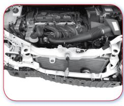
7.2.J Good example. Bonnet landing panel set back from the front bracket, avoiding subsequent damage.
