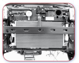
7.2.G Good example. The front panel comprises a landing panel but no lower parts. Costly parts set back enough to reduce damage.
