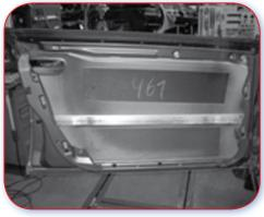
Good Example. Good accessinility for panel beating operations. The side impact protection bar is mounted by bolts, so it is possible to remove it to improve the accessibility.
