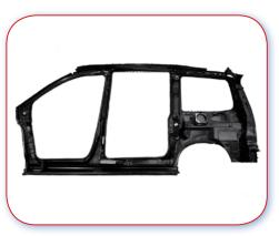
16.1.C Good example. Service parts supplied as a whole that can be cut where required to suit the damage to the vehicle. This avoids any mismatching joints.
