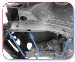
Good Example. Front chassis leg with a central data point, offering an additional reference for pulling operations.
