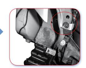
7.2.E Good example. On impact the panel has broken, allowing parts fitted to the panel to move but not to be damaged.
