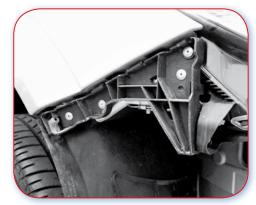
1.1.D Poor example. Bracket is supporting the panel and bumper independently. Fastener for the panel is covered by the bracket.
