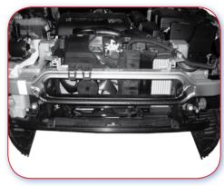
2.1.B Good example. Parts clip onto the bumper beam for easy release.
