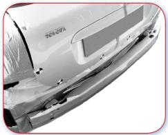
22.0.A Beam has been pushed forward, deforming the rear panel slightly.
