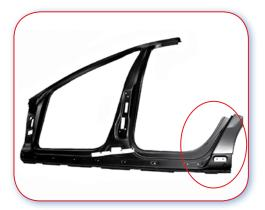
16.1.G Poor example. Service parts supplied as a side panel segment but having a joint at one of the most vulnerable and most frequently damaged parts like the dog leg.
