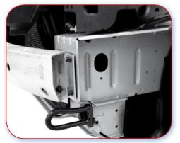
3.0.B Poor example. No crush can, so the chassis leg will be damaged on impact.
