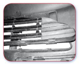
1.6.A Good example. Bumper grille can be removed for refit of new bumper.
