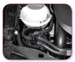
C.4.1 Poor example. Expensive auxiliary units positioned in vulnerable areas.
