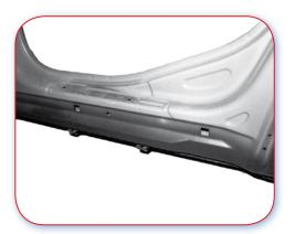
13.4.B Good example. Sill cover panel runs from edge to edge over the reinforcement around the 'B' Post and rear reinforcement.
