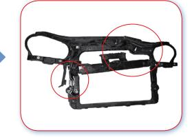
7.2.B Good example. On impact, the panel has broken, allowing parts fitted to the panel to move, but not to be damaged.
