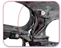
7.2.C Good example. Detail of damage to offer up panel.
