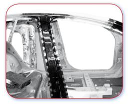
13.0.D 'B' Post cannot be sectioned so the roof rail has to be opened to allow the 'B' Post panel with its 'non-weldable' press hardened reinforcement, to be fitted onto the roof rail and sill.
