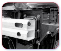
3.0.A Poor example. No crush can, so the chassis leg will be damaged on impact.
