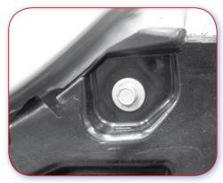
Good Example. Plastic element fixed with screws. Removing the screws is easy and causes no additional problems.
