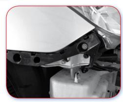
1.1.A Good example. Bracket is supporting the panel and bumper independently.
