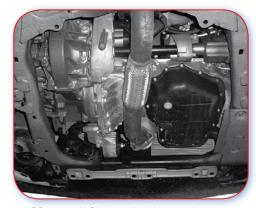
10.0.E Poor example. Single round sub-frame, any damage means complete replacement will be required.
