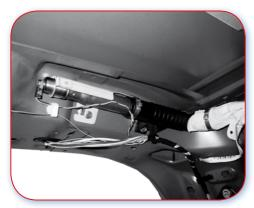
17.4.B Good example. As the curtain airbag generator is fitted onto the upper roof joint, removal is not required during repair.
