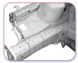
4.1.C Good example. These panels are set back, leaving space for light clusters and the front panel to move. Panels have natural joints to work to for removal of the part when damaged.
