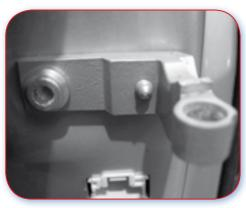
Poor Example. The limited access through holes in the door frame causes problems in repair.
