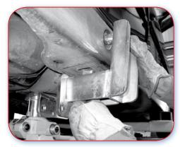
Poor Example. Sill panel without longitudinal flange implies the use of a special anchoring system.
