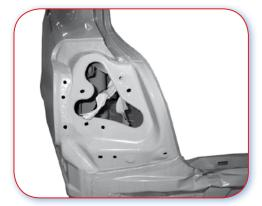
17.2.A Poor example. Rear quarters built up from several parts cause difficulty when separating and aligning parts in repair.
