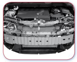
2.1.A Good example. Good distance between reinforcement and cooling pack. Good reinforcement height and no parts clip onto it.
