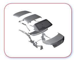
15.4.A Poor example. Folding roof assembly consisting of more then three panels.
