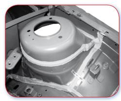
5.3.A Good example. Suspension strut tower, separate from the plenum chamber, showing joints to work to for replacement.
