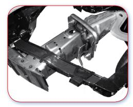
3.0.F Good example. A bolt-on crush can. This is a long crush can made from steel.
