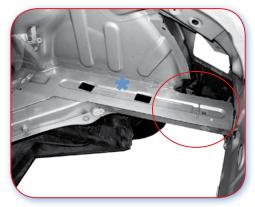
20.3.E There is enough space on the leg to deform in an impact, and enough space between the leg and wheel arch to remove the leg.\*
