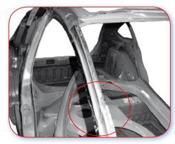
12.0.B Good example. 'A' post reinforcement is sectionable at natural joint in upper part, avoiding complete removal.
