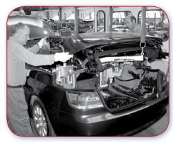
15.1.A Poor example. Removal of the complete roof in stowed position is difficult due to the shape and available space.
