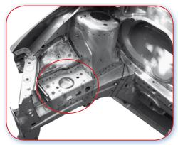
9.1.A Poor example. Small chassis leg with bracketing and holes not offering a good location for sectioning.
