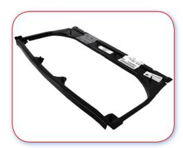
19.0.B Good example. Boot floor area in BIW without reinforced plastic infill and service repair part.
