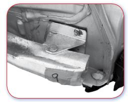
21.0.C Good example. A bumper beam fitted on crush cans absorbs energy on impact and creates space for deformation.
