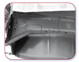
20.1.A Good example. Chassis leg is sectionable on a natural joint. This will improve ease of repair.
