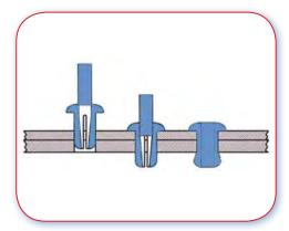
C.10.1 An example of poor clips. Pin will be lost on removal.
