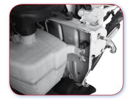
3.0.E Poor example. No crush can for energy absorption, leaving the chassis leg to be damaged on impact.
