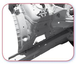
4.1.H Good example. No inner wing, just a reinforcement joining the panel reinforcement and chassis leg. An arch lining forms the joint between the front panel, inner wing and panel reinforcement.
