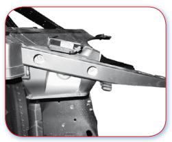
12.1.C Good example. Side panel reinforcement bolted onto plenum chamber/'A' Post. This will ease the replacement.
