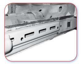
13.5.C Good example. Sill reinforcement is made of separate parts and can be repaired by partially removing the sill reinforcement.
