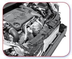
7.2.D Good example. Bolt-on front panel made out of reinforced plastic.
