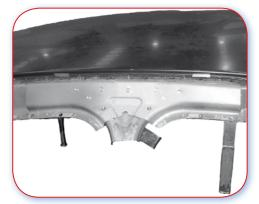
13.2.F Poor example. 'B' Post has to be sectioned and roof rail has to be opened for the reinforcement to be fed between panels.
