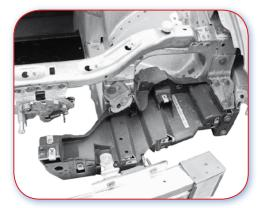
7.1.A Poor example. Front panel welded to side member.
