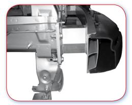
3.0.G Good example. A bolt-on crush can. This is a short crush can made from aluminium.
