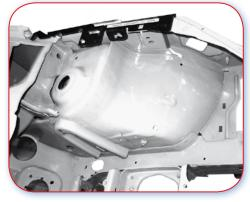
5.2.A Poor example. Suspension strut tower is positioned as part of the firewall plenum chamber.
