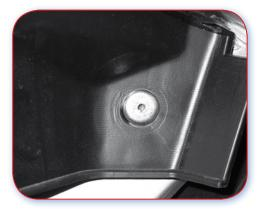
Poor Example. Plastic element fixed with rivets. Removal of the rivets could damage it.
