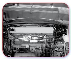
15.3.B Good example. The complete assembly, including electro hydraulic system, can be removed.
