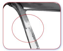
12.0.C Good example. 'A' Post reinforcement is sectionable at natural joint in upper part, avoiding complete removal.
