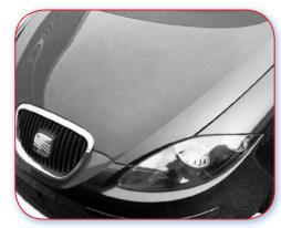
8.1.B Good example. Front edge of bonnet set back. Side edges protected by side panel.
