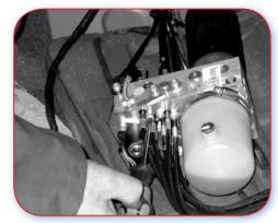
15.3.A Poor example. Hydraulic system to be drained before separation of the system from the folding roof.
