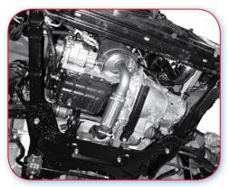
10.0.A Good example. Sub-frame segmented, any damaged parts can be easily replaced.
