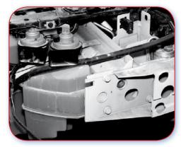
9.1.1 Poor example. Chassis rail does not have crush cans incorporated in bumper system.
