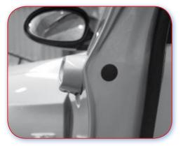
Poor Example. A doorskin with the curvature inwards makes it difficult to repair and paint.
