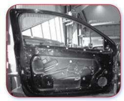
Poor Example. The limited access through holes in the door frame makes repair difficult.
