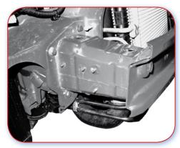
3.0.J Good example. Good space between bar and cooling pack. This is an average length crush can made from steel.
