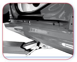
13.5.A Sill shape is given by fitting a plastic cover in the body colour.
