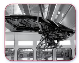
15.2.B Good example. Appropriate lifting tool reduces the number of people required and reduces risk of damage.
