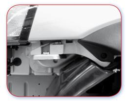
1.1.C Poor example. Bracket to carry bumper is fitted to panel.
