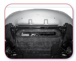
11.3.A Good example. Under tray covering engine bay, fixed with hexagonal head screws, not breakable clips or staples.
